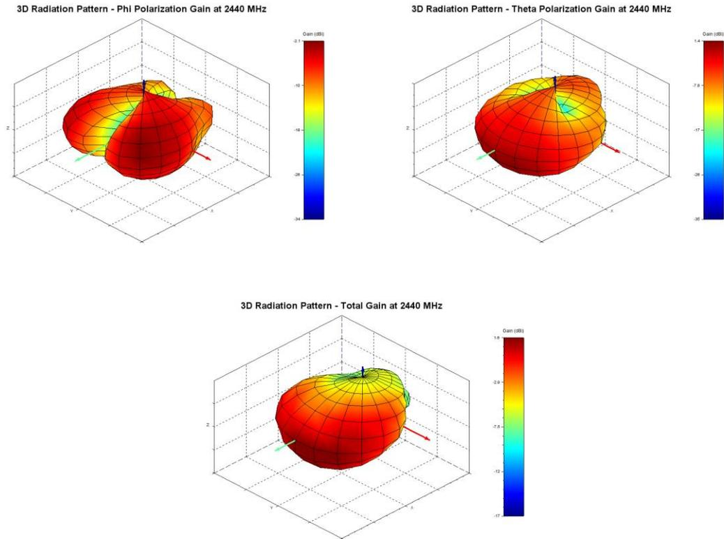
**Figure 8: Phi, theta, and total gain plots – 2440 MHz**
