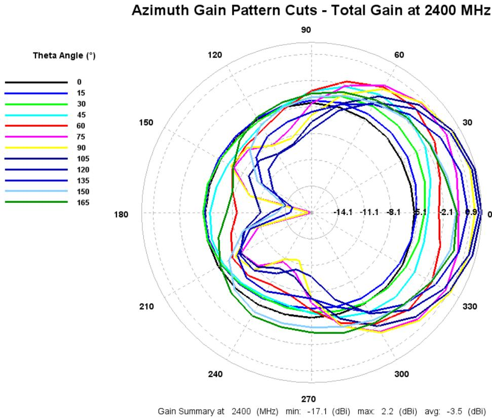
**Figure 5: Total gain pattern – 2400 MHz**
