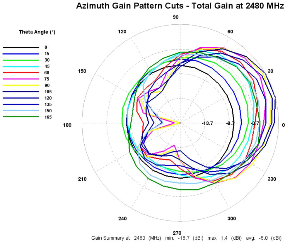
**Figure 9: Total gain pattern – 2480 MHz**
