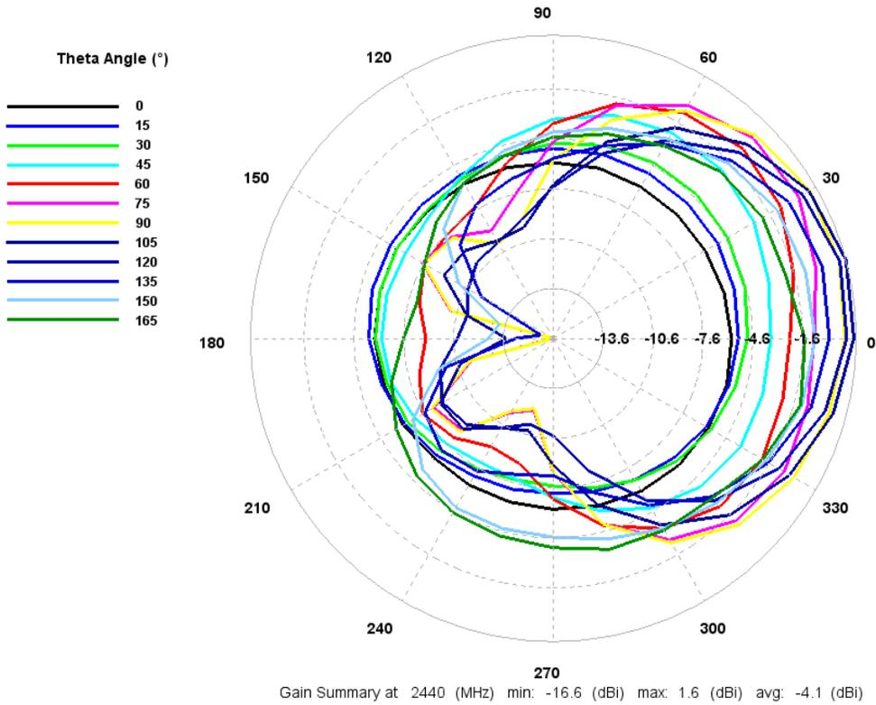
Figure 7: Total gain pattern – 2440 MHz
