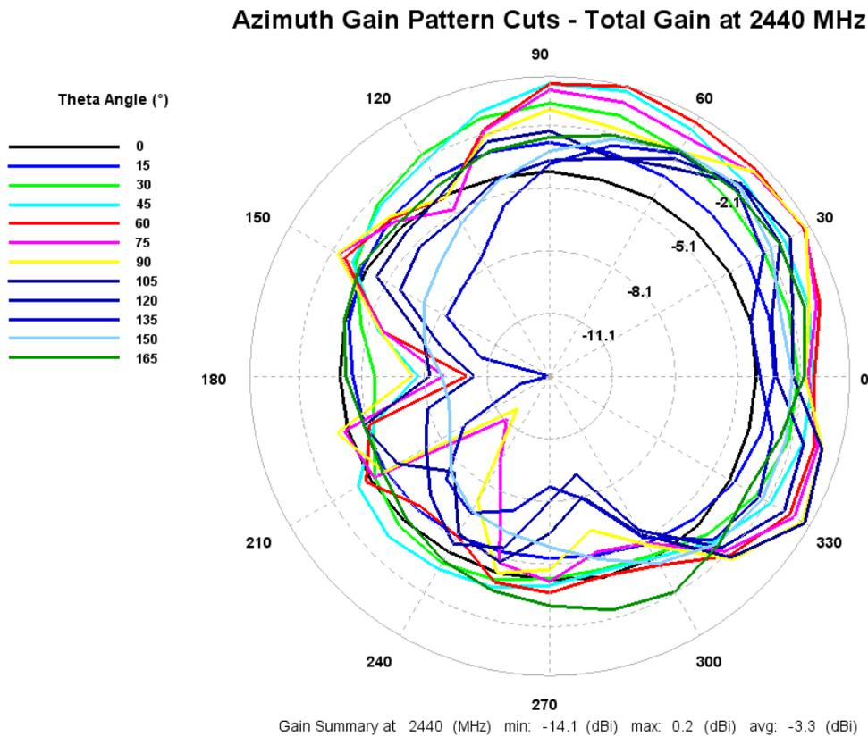
**Figure 12: Total gain pattern – 2440 MHz**
