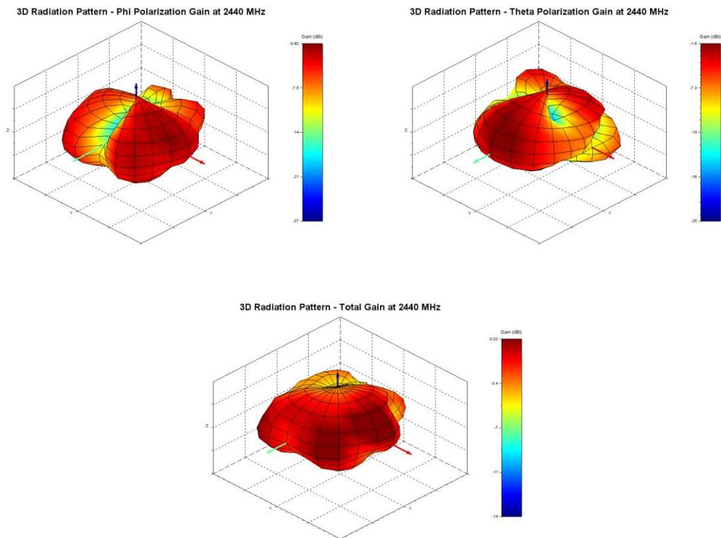
**Figure 13: Phi, theta, and total gain plots – 2440 MHz**
