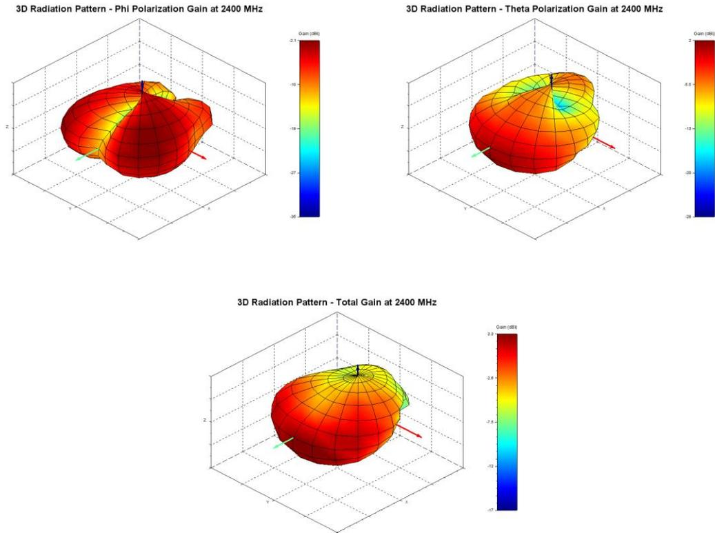
**Figure 6: Phi, theta, and total gain plots – 2400 MHz**
