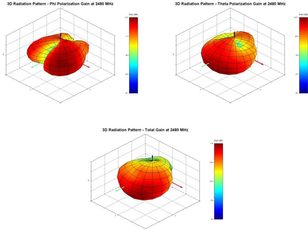
**Figure 10: Phi, theta, and total gain plots – 2480 MHz**
