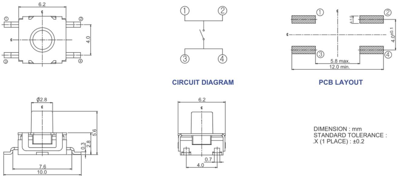
**Figure 2 – 222PJV, Surface Mount J Bend, Actuator Height 5.6mm**
