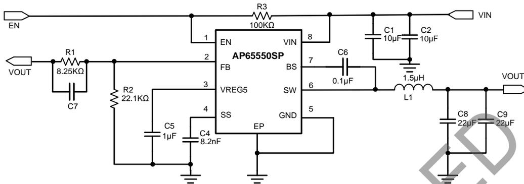
**Figure 3 Typical Application of AP65550SP (SO-8EP) Evaluation Board**
