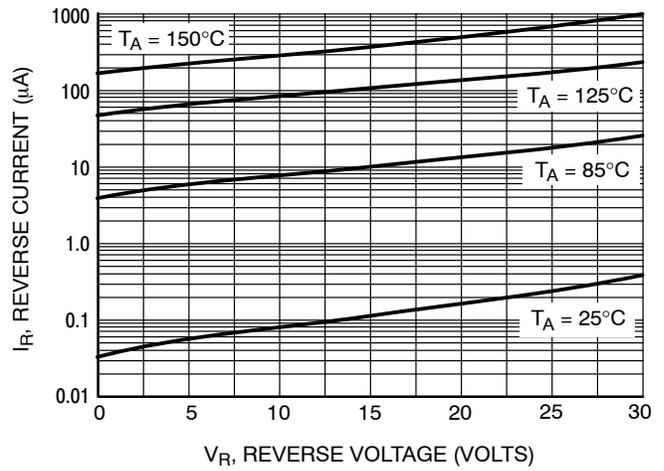
**Figure 3. Leakage Current**
