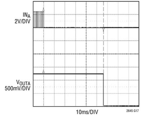
**Entering Idle Mode Full-Scale From Mid-Scale (IDLSEL = GND)**
