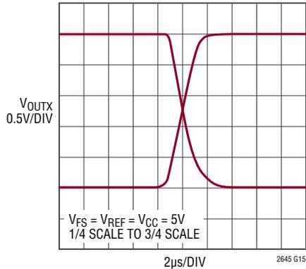
**$IN_X$  to  $V_{OUTX}$  Delay Full-Scale Transition**
