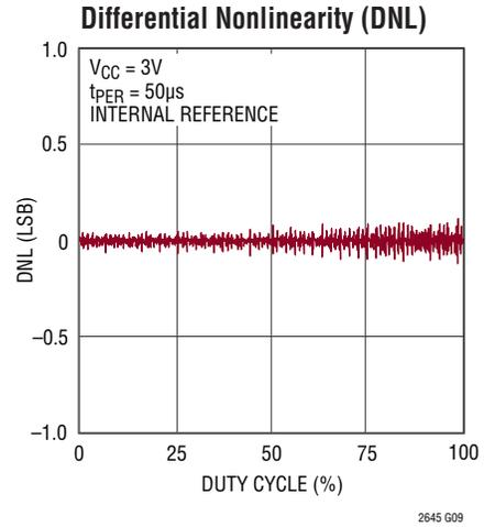
LTC2645-8 (Internal Reference, V<sub>FS</sub> = 2.5V)
