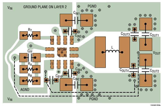
(b) With Capacitors  $C_{OUT1}$  and  $C_{OUT2}$  Rotated by  $90^\circ$ , Which Reduces High Frequency Output Ripple. Optional 0201 Capacitors  $C_{OUT3}$  and  $C_{OUT4}$  Further Improve the High Frequency Output Ripple. Five 5mil Vias Are Used within the EPAD. For Layouts Where 5mil Vias Are Not Allowed, It Is Recommended to Use Either Four 8mil Vias or a Single (Filled or Tented) 12mil Diameter Via.
