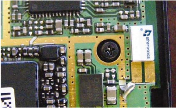
Ethertronics' Savvi series of Isolated Magnetic Dipole™ (IMD) antennas deliver on the key needs of device designers for higher functionality and performance in smaller/thinner designs. These innovative antennas provide compelling advantages for Bluetooth® enabled cell phones, media players and other mobile devices.
