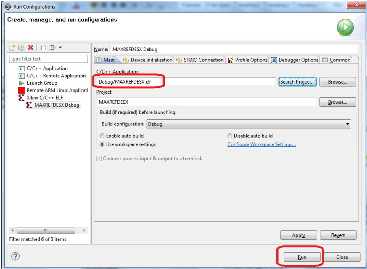
Once the Debug/MAXREFDES12 configuration is set up once, you just need to press the **Run** button if you ever want to run the program again.
