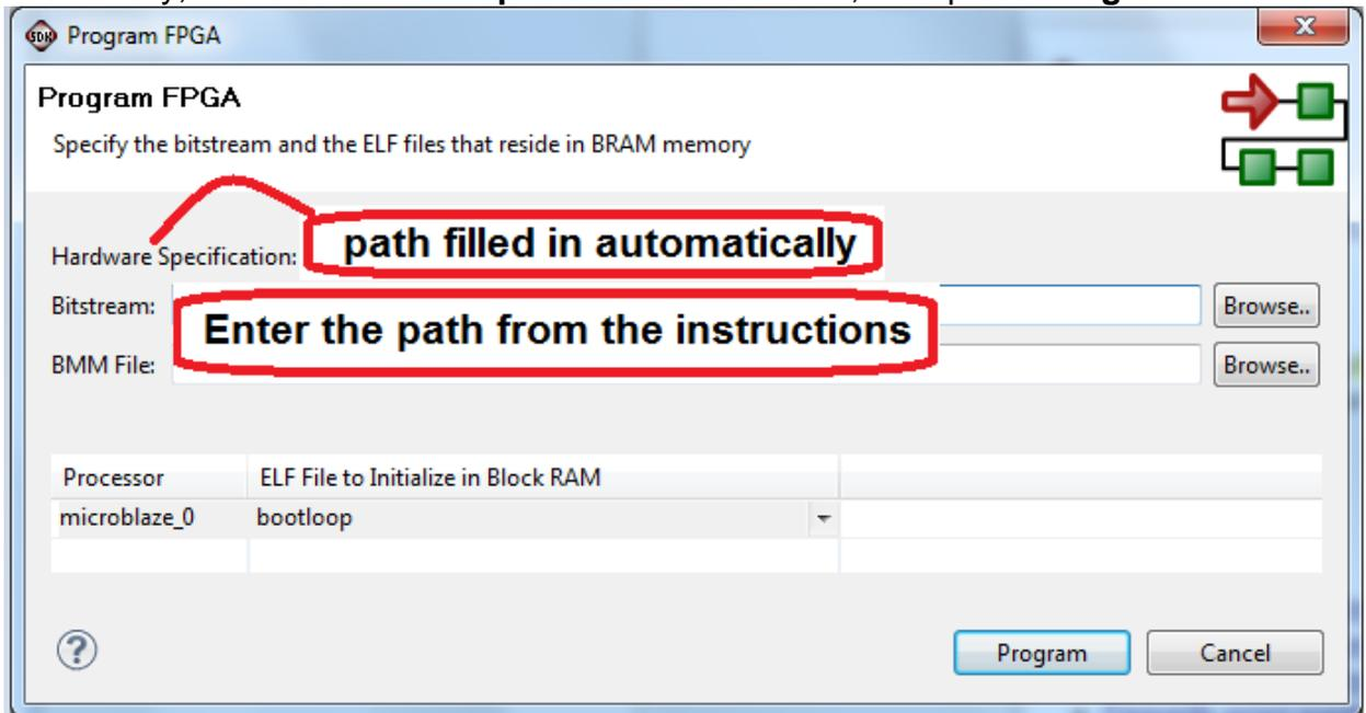
It takes approximately 10 seconds to download the FPGA, then a message box indicating **FPGA configuration complete** appears.
