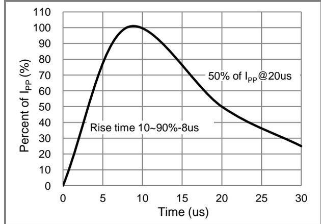
Fig.2 Pulse Waveform
