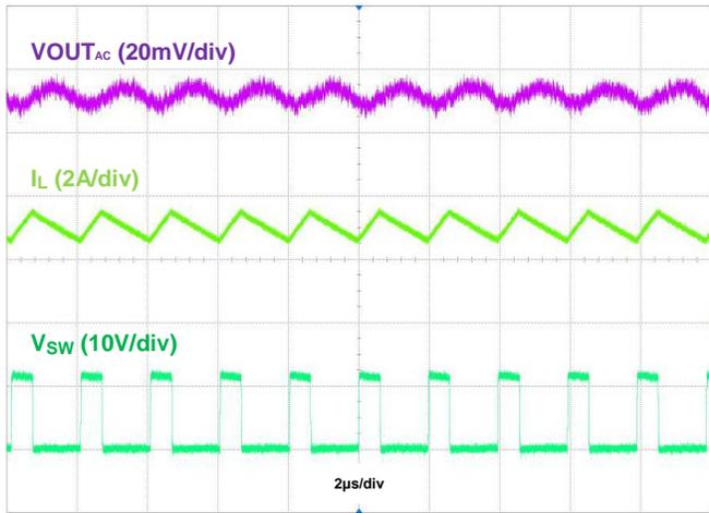
Figure 23. Output Ripple,  $V_{IN}=12\text{V}$ ,  $V_{OUT} = 3.3\text{V}$  @3A, PFM
