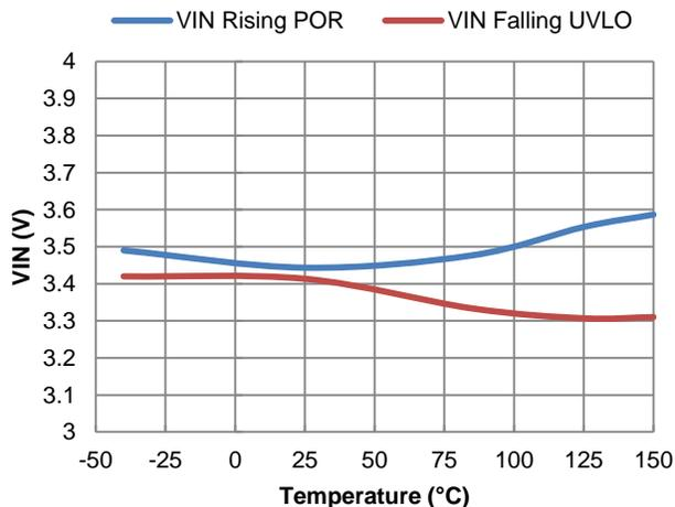
Figure 9. VIN POR and UVLO vs. Temperature
