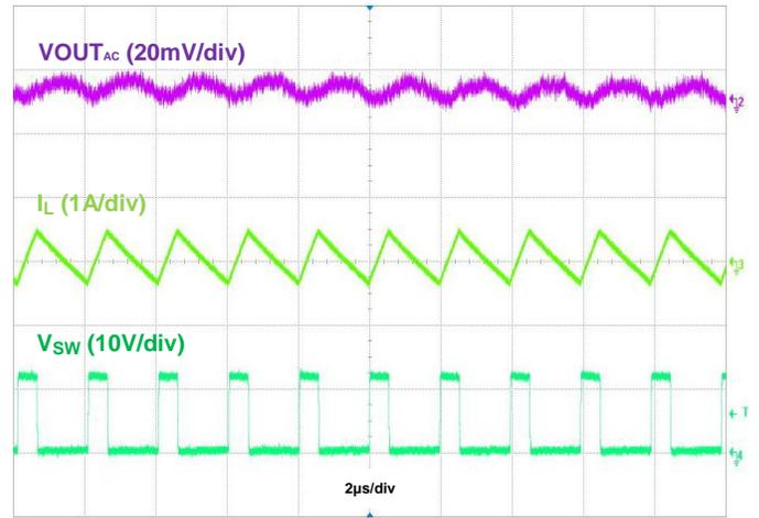
Figure 24. Output Ripple,  $V_{IN}=12\text{V}$ ,  $V_{OUT} = 3.3\text{V}$  @50mA, PFM
