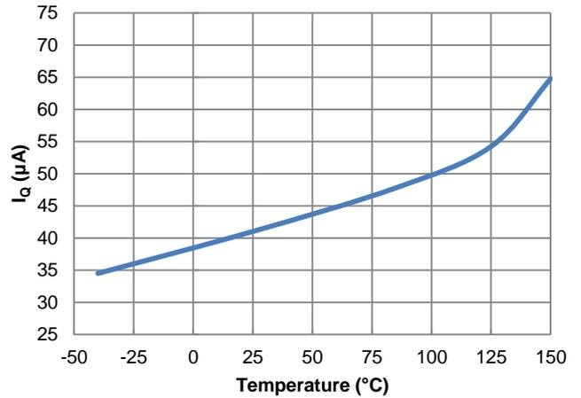
Figure 12.  $I_q$  vs. Temperature,  $I_{OUT} = 0\text{A}$
