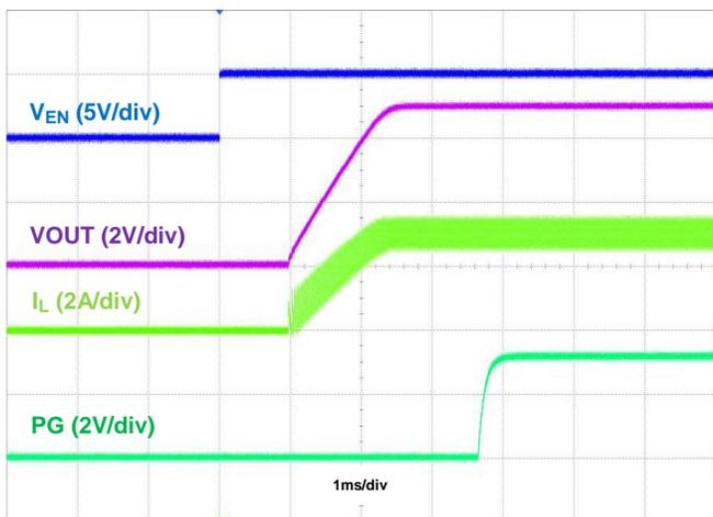
Figure 33. Startup using EN with PG, IOUT = 3A
