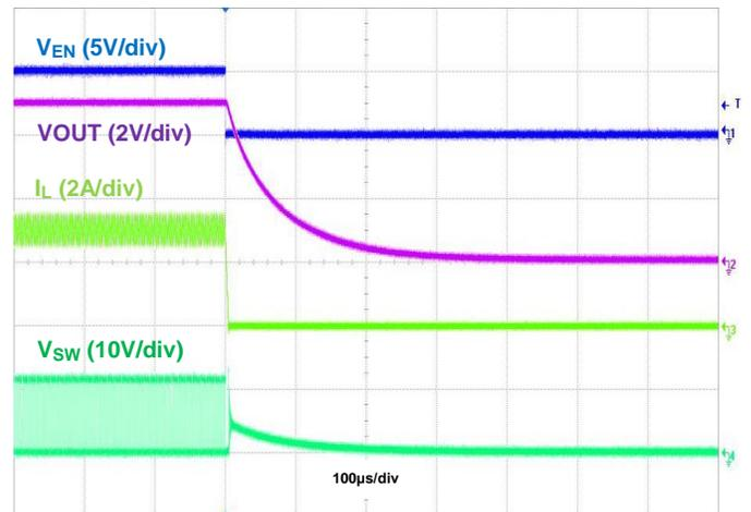
Figure 32. Shutdown using EN, IOUT = 3A
