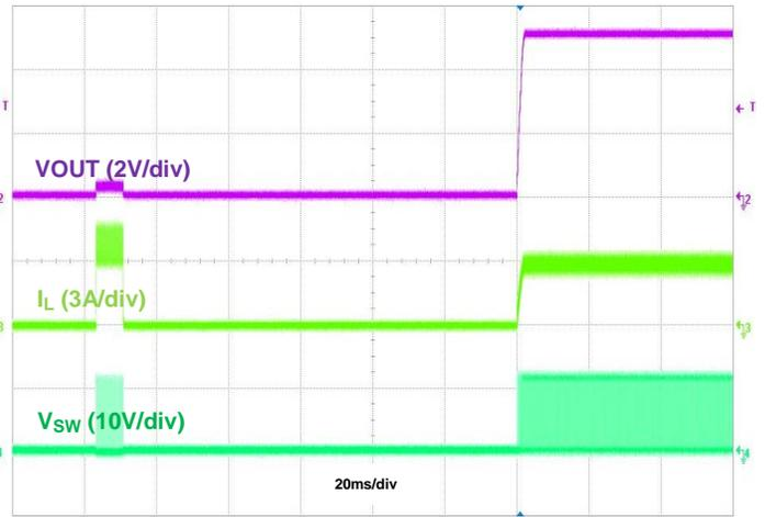
Figure 36. Output Short Recovery,  $I_{OUT} = 3\text{A}$
