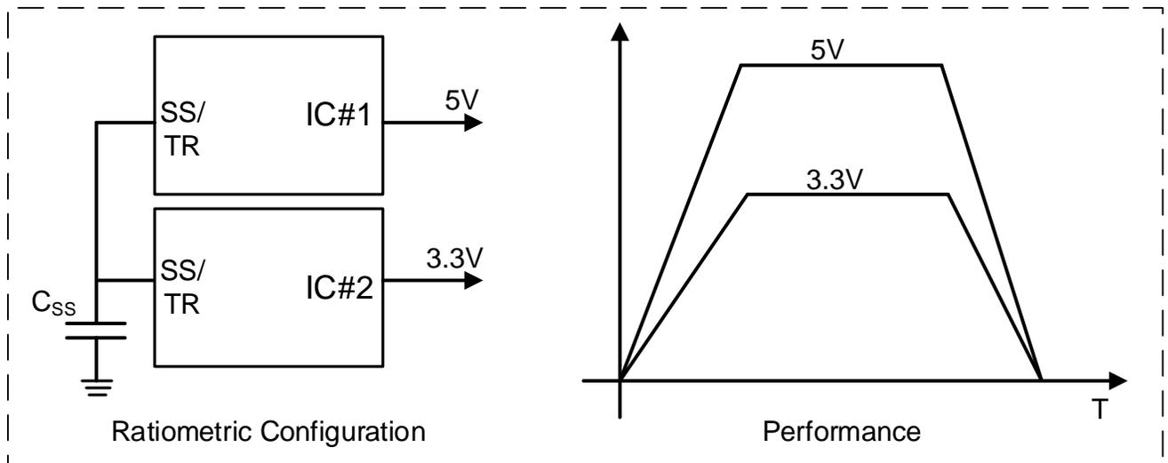
**Figure 37. Ratiometric Configuration**
