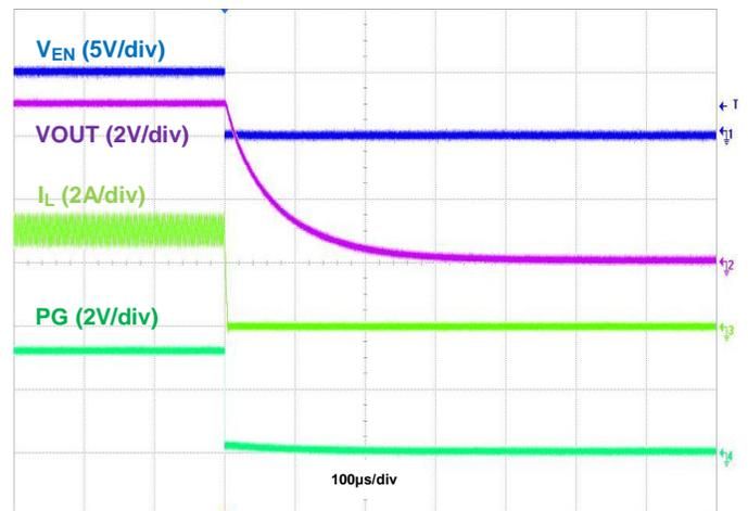
Figure 34. Shutdown using EN with PG, IOUT = 3A
