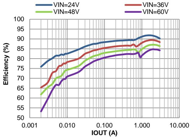
Figure 5. PFM Efficiency vs. Output Current,  $V_{OUT}=5\text{V}$ ,  $L=6.5\mu\text{H}$
