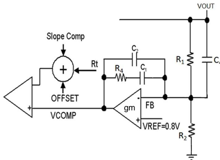
Figure 46. Type 2 Compensator
