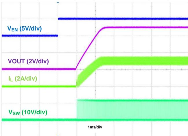
Figure 31. Startup using EN, IOUT = 3A
