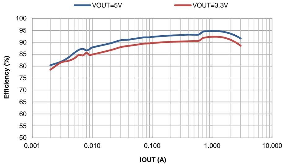
**Figure 2. PFM Efficiency vs. Output Current, VIN = 12V, f<sub>sw</sub> = 500kHz**
