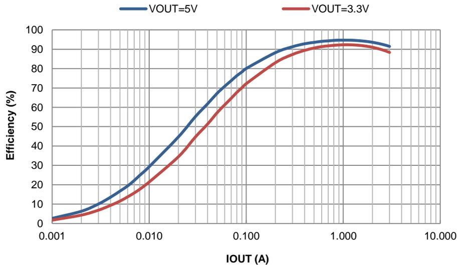
**Figure 3. PWM Efficiency vs. Output Current, VIN = 12V, f<sub>sw</sub> = 500kHz**
