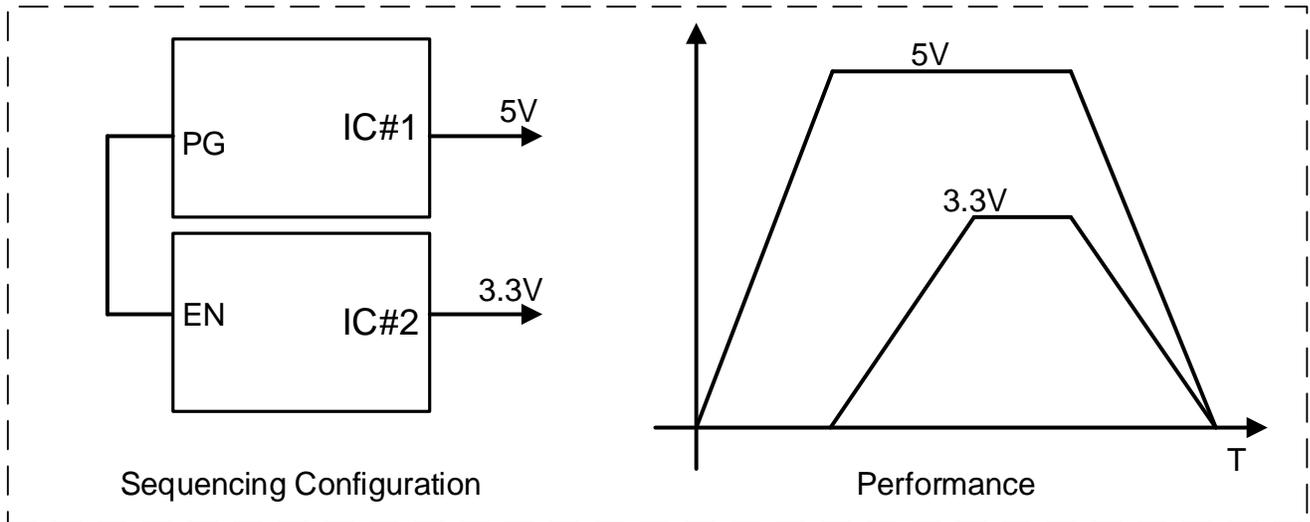
Figure 39. Sequencing Configuration
