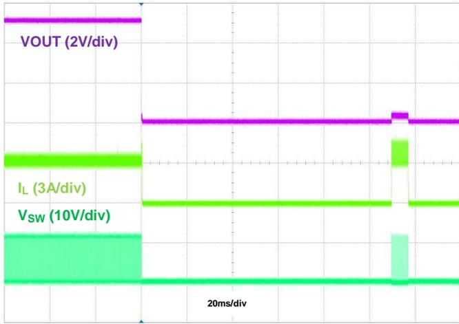
Figure 35. Output Short Protection,  $I_{OUT} = 3\text{A}$
