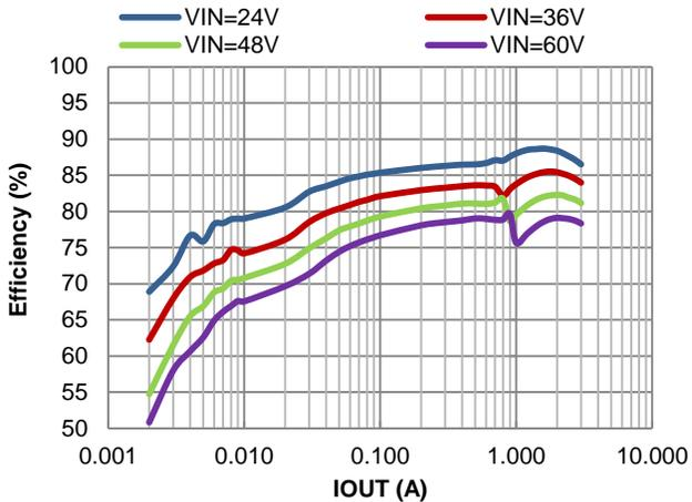
Figure 7. PFM Efficiency vs. Output Current,  $V_{OUT}=3.3\text{V}$ ,  $L=5.5\mu\text{H}$
