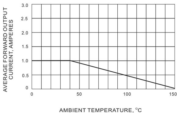
FIG. 1 DERATING CURVE FOR OUTPUT RECTIFIED CURRENT
