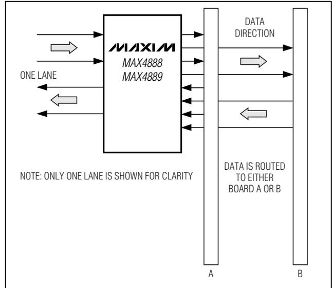
Figure 5. The MAX4888/MAX4889 Used as a Single-Lane Switch
