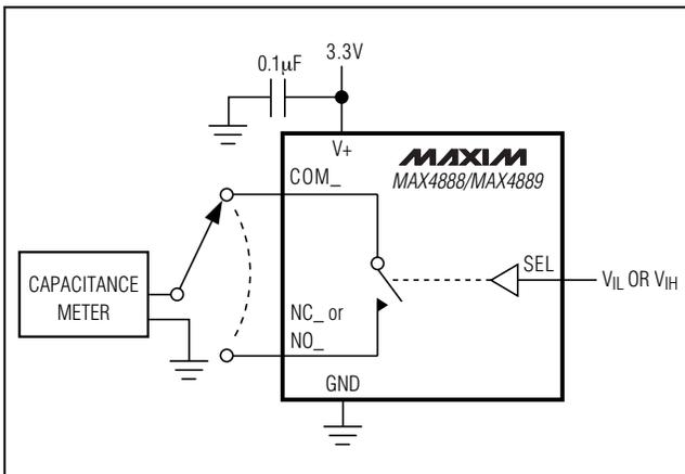
Figure 4. Channel Off-/On-Capacitance
