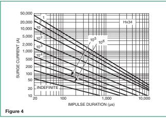
NOTE: If pulse ratings are exceeded, a shift of  $V_{NDC_1}$  (at specified current) of more than +/-10% could result. This type of shift, which normally results in a decrease of  $V_{NDC_1}$ , may result in the device not meeting the original published specifications, but it does not prevent the device from continuing to function, and to provide ample protection.
