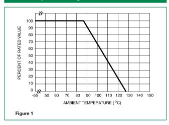
Should transients occur in rapid succession, the average power dissipation result is simply the energy (watt-seconds) per pulse times the number of pulses per second. The power so developed must be within the specifications shown on the Device Ratings and Specifications Table for the specific device. The operating values must be derated as shown in above.
