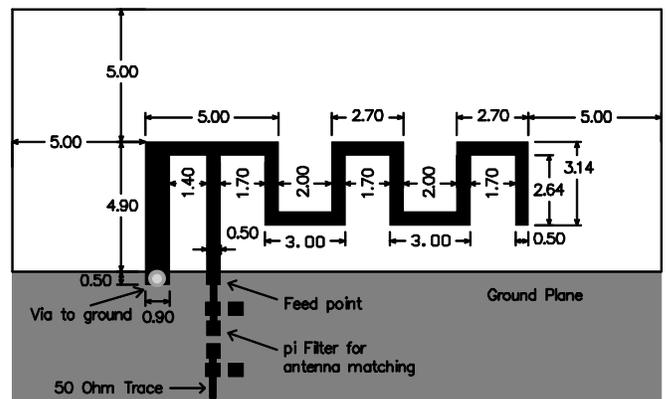
Figure 8 - Trace Antenna (dimensions in mm)
