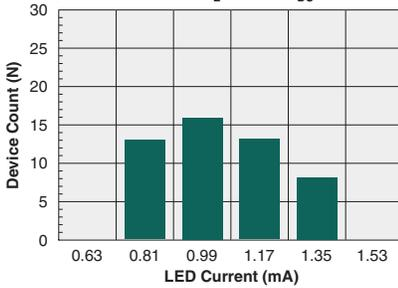
**Typical  $I_F$  for Switch Dropout**
