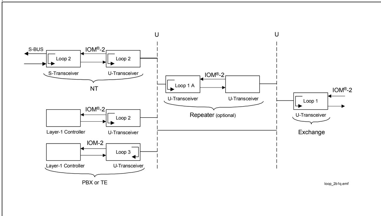
**Figure 49 Test Loopbacks**
