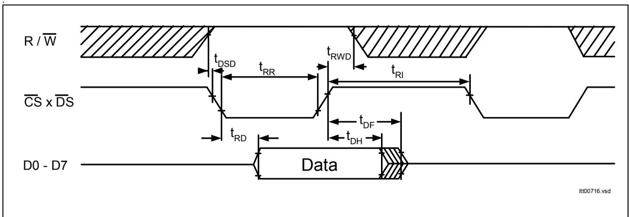
Figure 69 Microprocessor Read Timing
