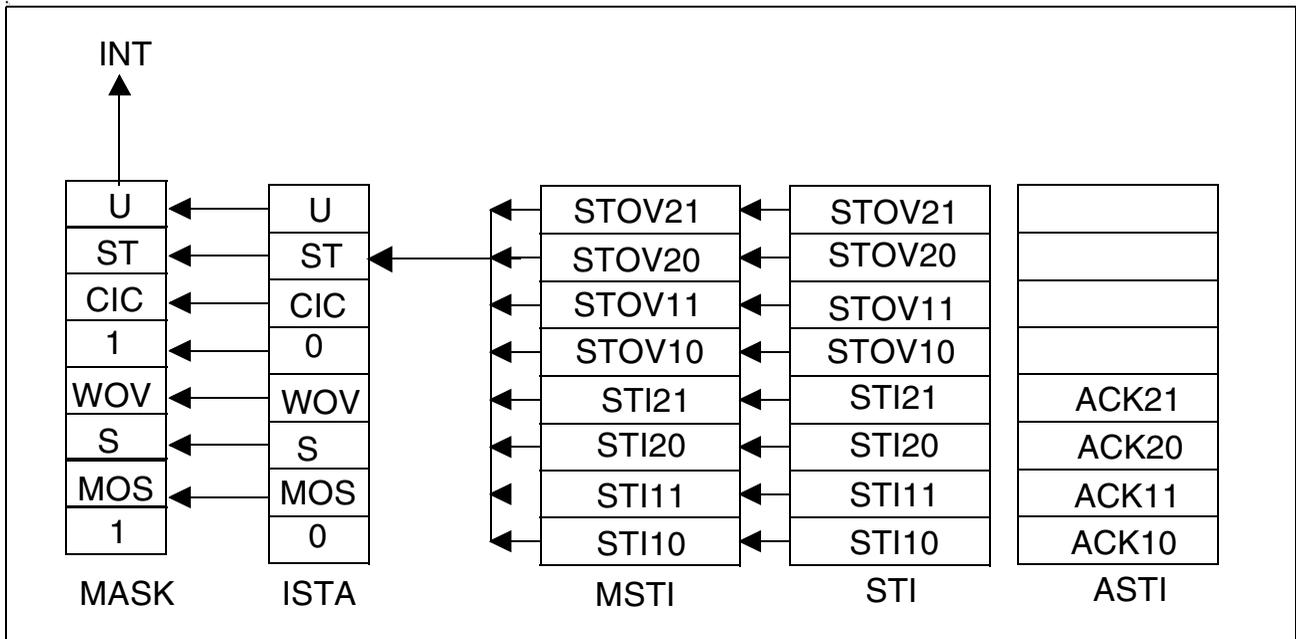
**Figure 17 Interrupt Structure of the Synchronous Data Transfer**
