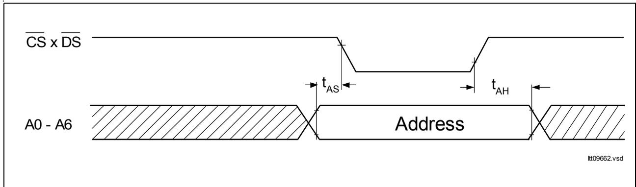
Figure 71 Non-Multiplexed Address Timing
