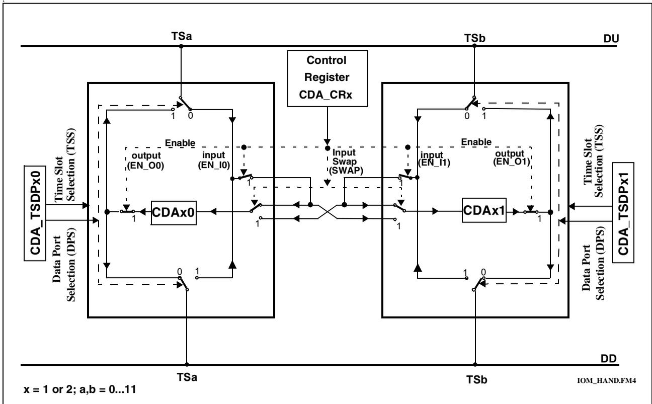
Figure 12 Data Access via CDAX0 and CDAX1 register pairs
