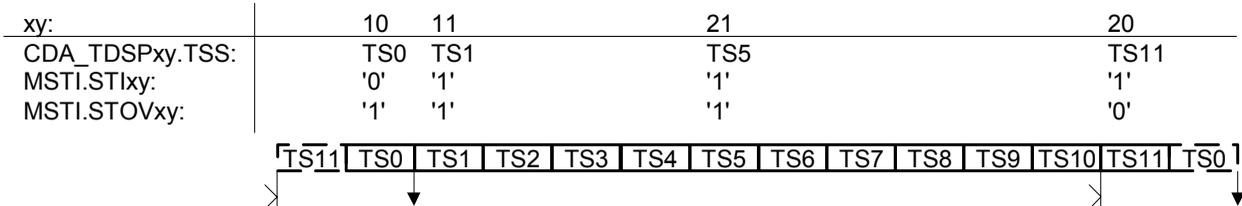
c) Interrupts for data access to time slot 0 and 1 (B1 and B2 after reset), MSTI.STI10, MSTI.STOV10, MSTI.STI11 and MSTI.STOV11 enabled
