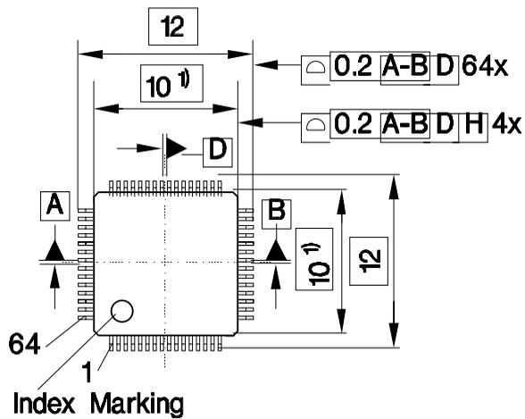
1) Does not include plastic or metal protrusion of 0.25 max. per side
