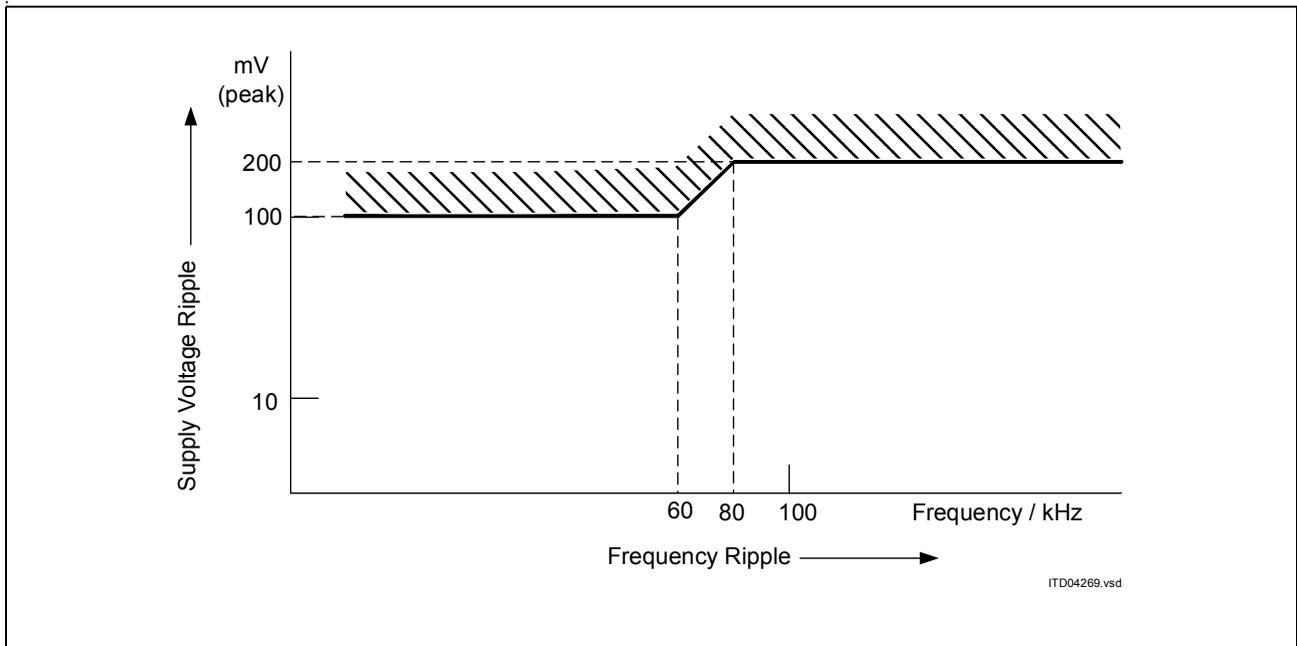
**Figure 60** Maximum Sinusoidal Ripple on Supply Voltage
