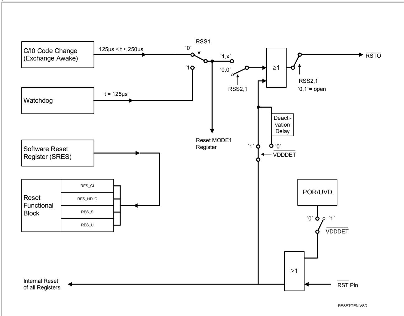
Figure 9 Reset Generation of the T-SMINT® I<sup>1)</sup>
