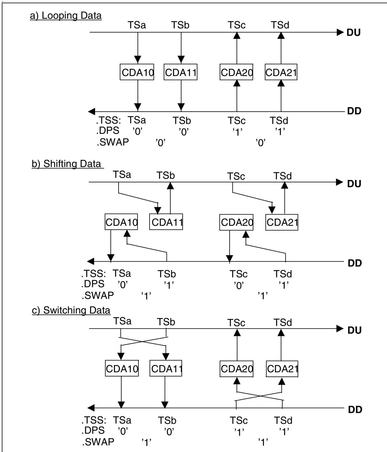
**Figure 13 Examples for Data Access via CDAxy Registers**
