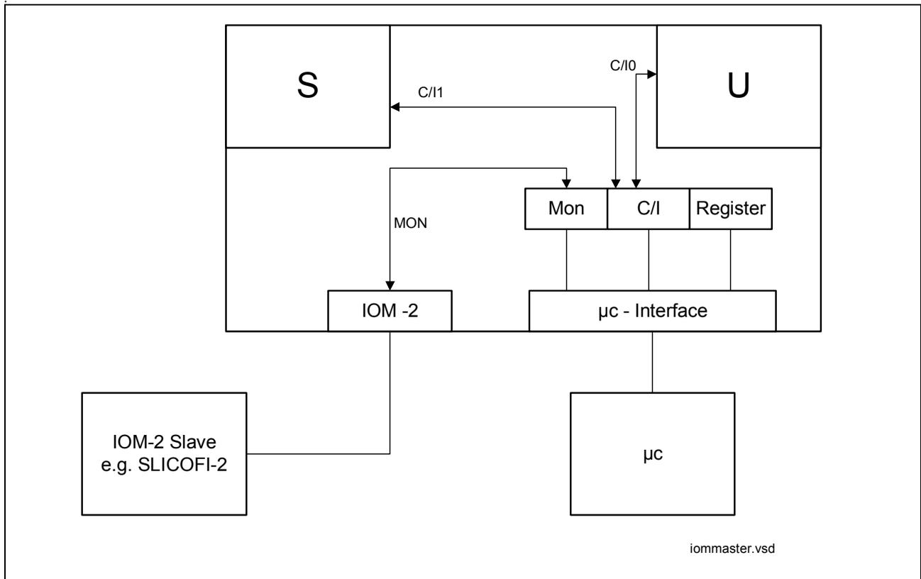
**Figure 4 Control via μP Interface**
