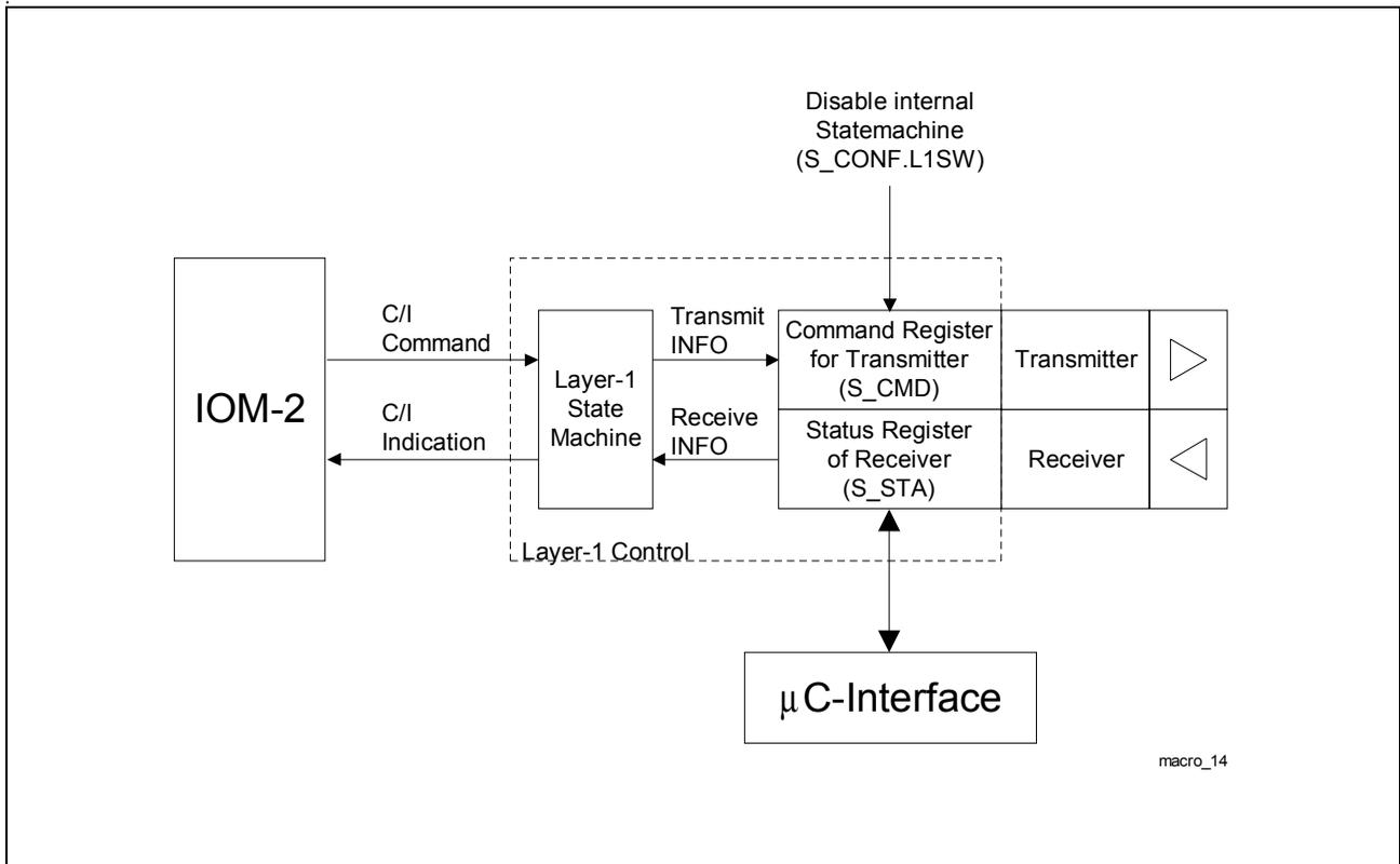
**Figure 39 S-Transceiver Control**
