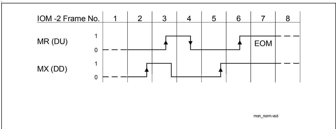
**Figure 23 Monitor Channel, Normal End of Transmission**
