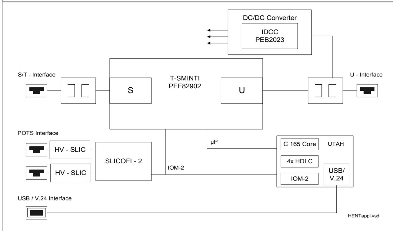
**Figure 3 Application Example T-SMINTI®: High Feature Intelligent NT**
