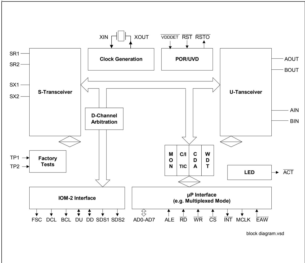
Figure 2 Block Diagram
