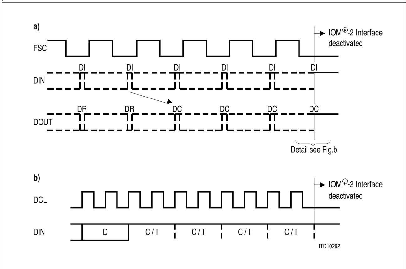
**Figure 31 Deactivation of the IOM<sup>®</sup>-2 Clocks**
