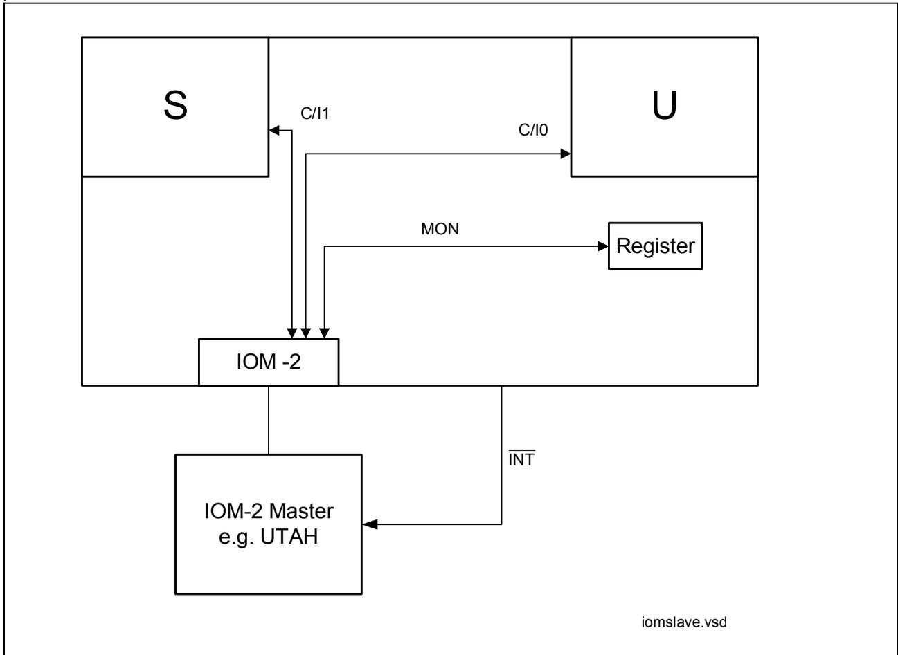
Figure 5 Control via IOM<sup>®</sup>-2 Interface
