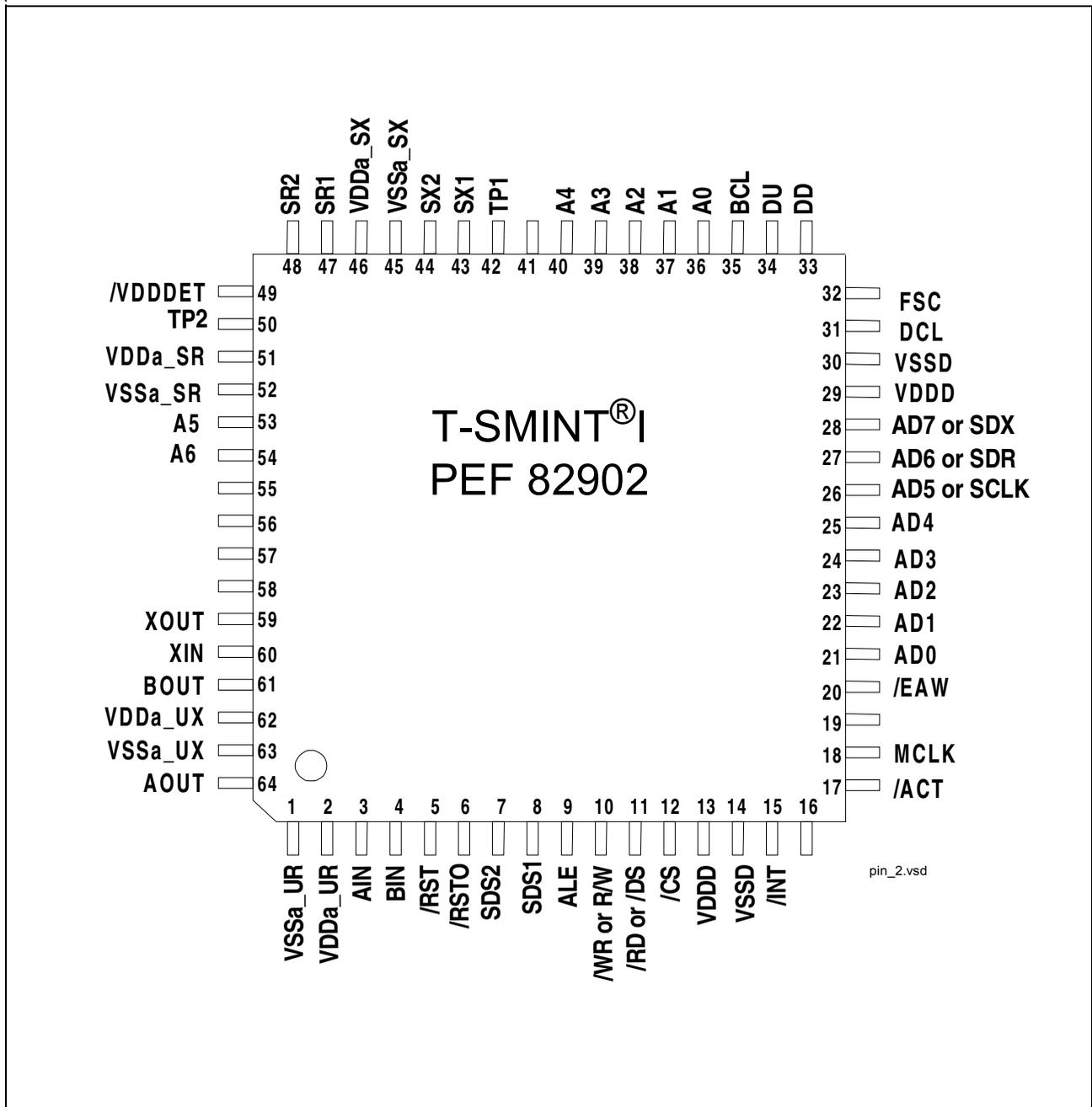
Figure 1 Pin Configuration
