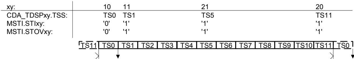
b) Interrupts for data access to time slot 0 (B1 after reset), STOV interrupt used as flag for "last possible CDA access"; MSTI.STI10 and MSTI.STOV20 enabled
