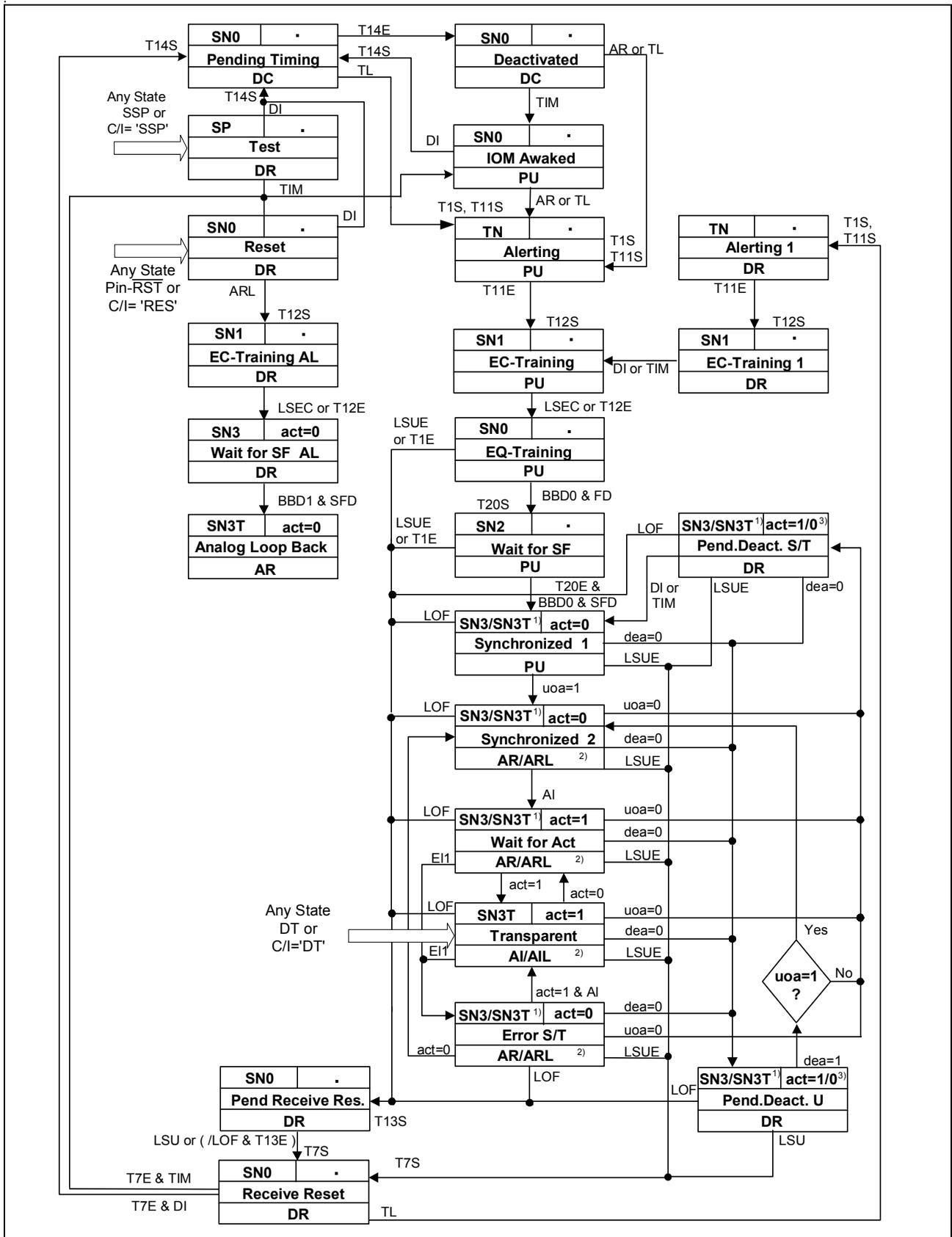
Figure 75 Simplified State Machine Q-SMINT® I: 2B1Q
