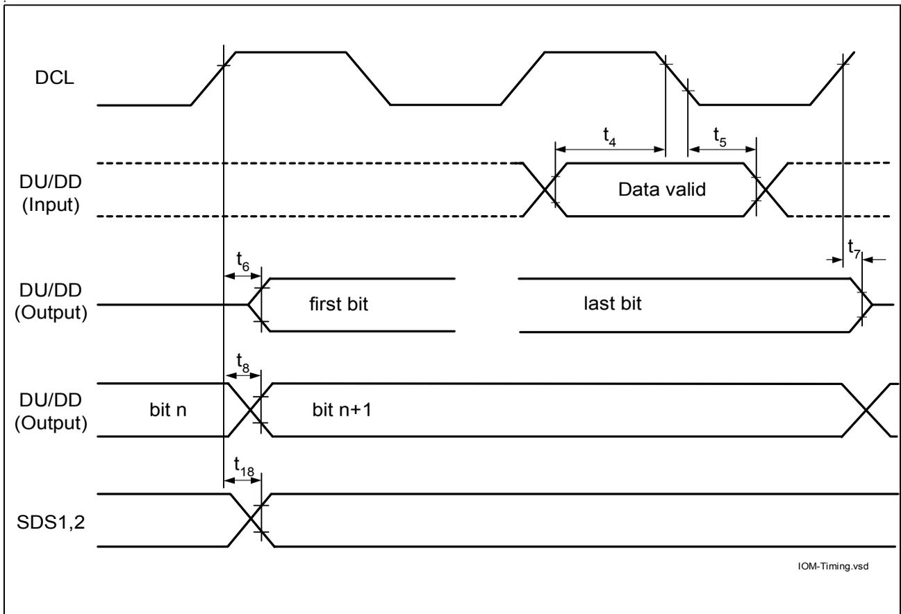
Figure 62 IOM<sup>®</sup>-2 Interface - Bit Synchronization Timing
