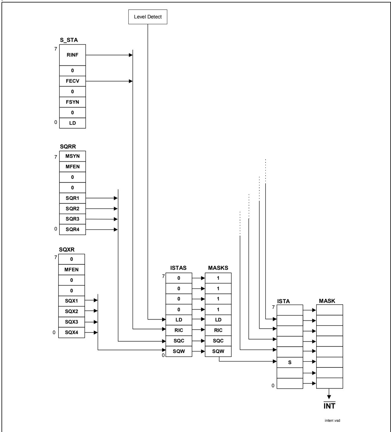
**Figure 43** Interrupt Structure S-Transceiver
