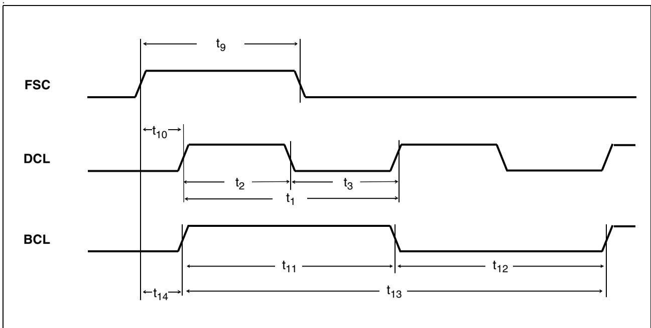
Figure 63 IOM<sup>®</sup>-2 Interface - Frame Synchronization Timing
