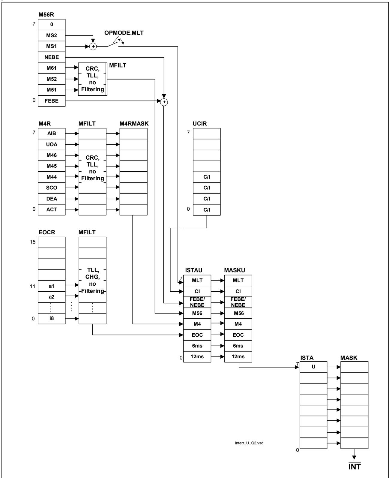
Figure 77 Interrupt Structure U-Transceiver Q-SMINT® I: 2B1Q
