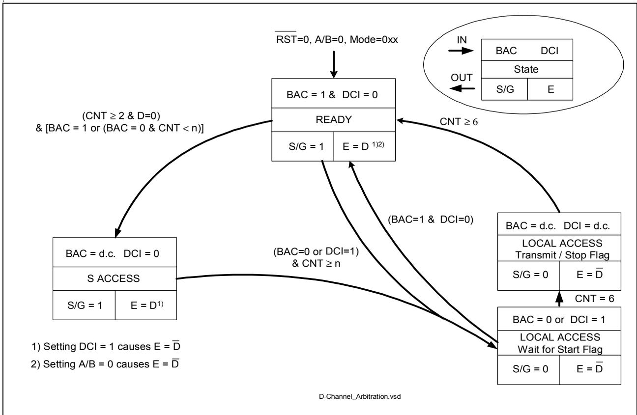
**Figure 30 State Machine of the D-Channel Arbiter (Simplified View)<sup>1)</sup>**
