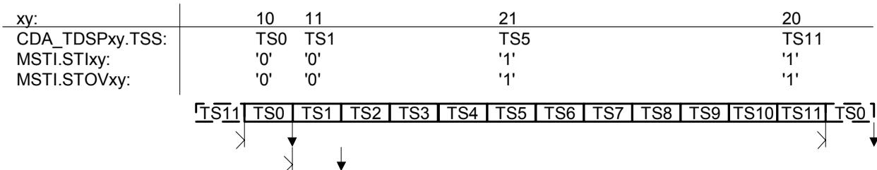
d) Interrupts for data access to time slot 0 (B1 after reset), STOV20 interrupt used as flag for "last possible CDA access", STOV10 interrupt used as flag for "CDA access failed"; MSTI.STI10, MSTI.STOV10 and MSTI.STOV20 enabled
