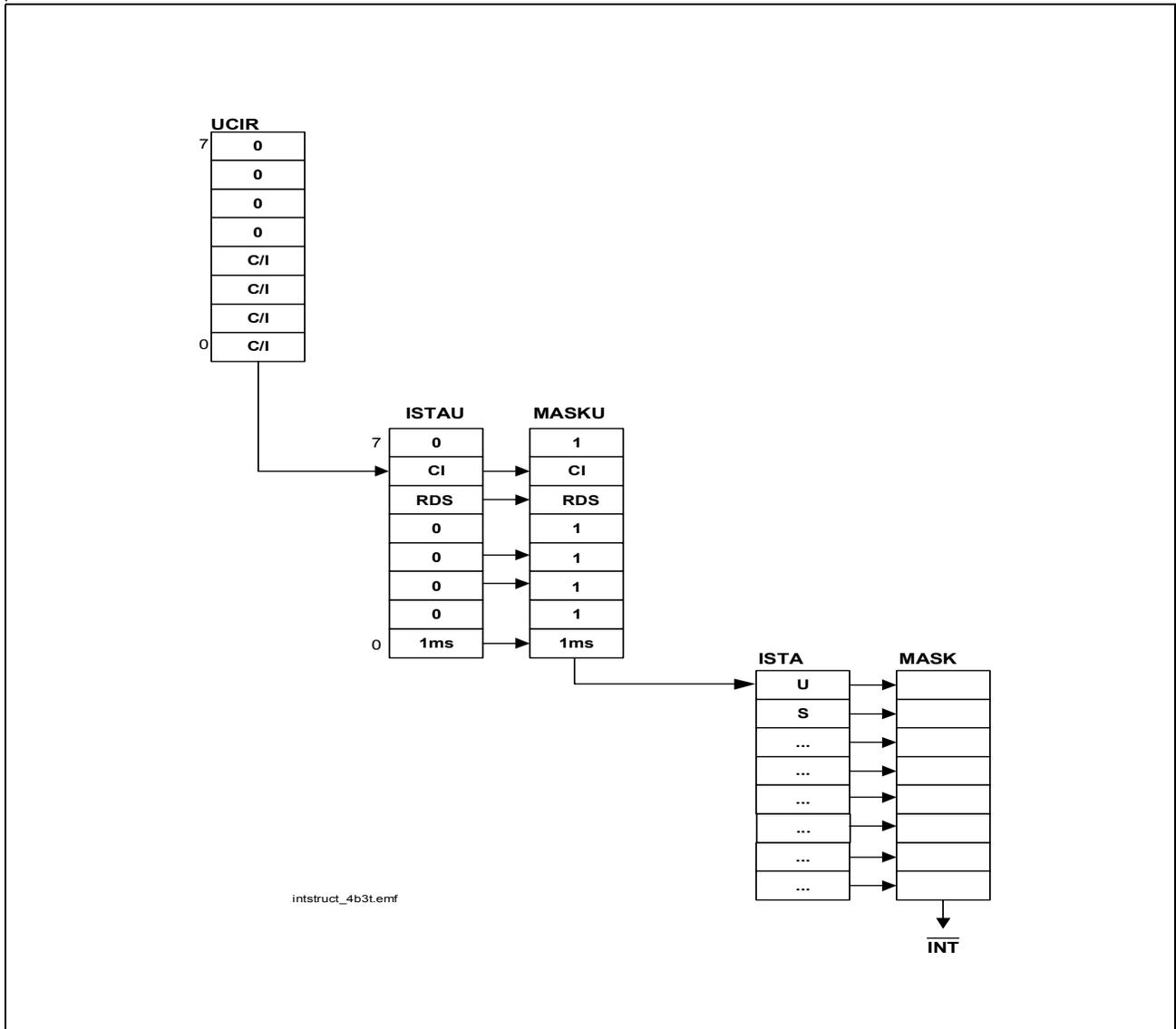
Figure 78 Interrupt Structure U-Transceiver T-SMINT® I: 4B3T
