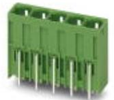
Header, Nominal current: 76 A, Rated voltage (III/2): 1000 V, Number of positions: 5, Pitch: 10.16 mm, Color: green, Contact surface: Silver, Assembly: Soldering
