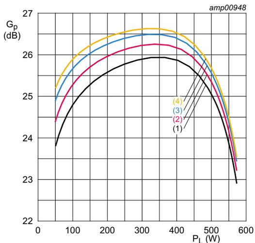
$V_{DS} = 50 \text{ V}; f = 433 \text{ MHz}; \text{CW.}$
