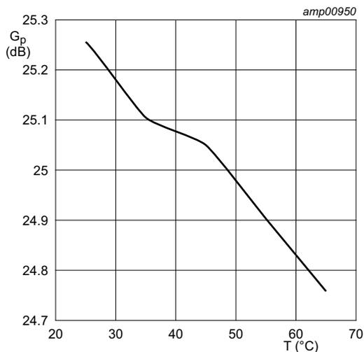
$V_{DS} = 50\text{ V}$ ;  $I_{Dq} = 50\text{ mA}$ ;  $f = 433\text{ MHz}$ ; CW; at  $P_{L(1dB)}$ .
