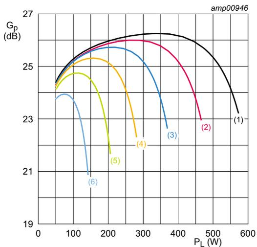
$f = 433 \text{ MHz}; I_{Dq} = 50 \text{ mA}; \text{CW.}$
