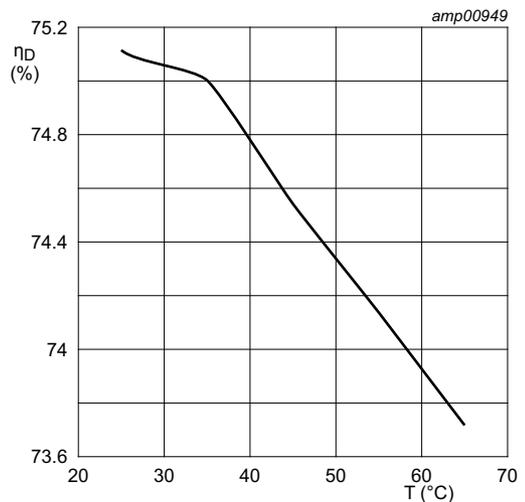
$V_{DS} = 50 \text{ V}; I_{Dq} = 50 \text{ mA}; f = 433 \text{ MHz}; \text{CW}; \text{at } P_{L(1dB)}$
