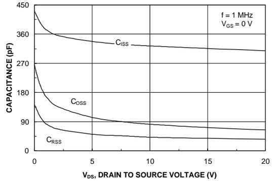
Figure 8. Capacitance Characteristics.
