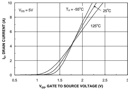
Figure 5. Transfer Characteristics.
