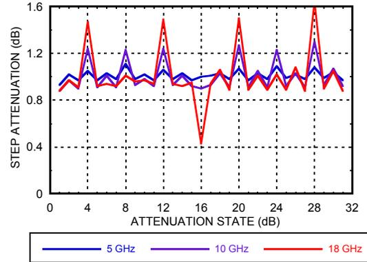
**Step Attenuation vs. Attenuation State**
