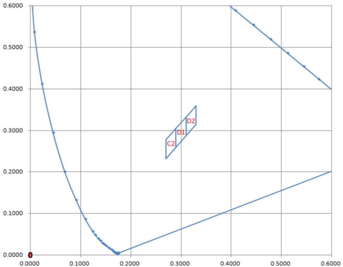
@5mA / Ta=25°C, It maintains a tolerance of x,y ± 0.007
