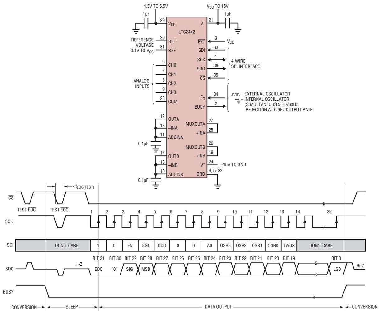
Figure 7. Internal Serial Clock, Single Cycle Operation
