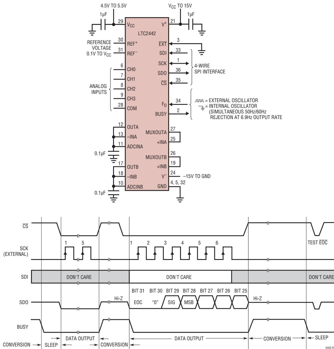
Figure 5. External Serial Clock, Reduced Output Data Length
