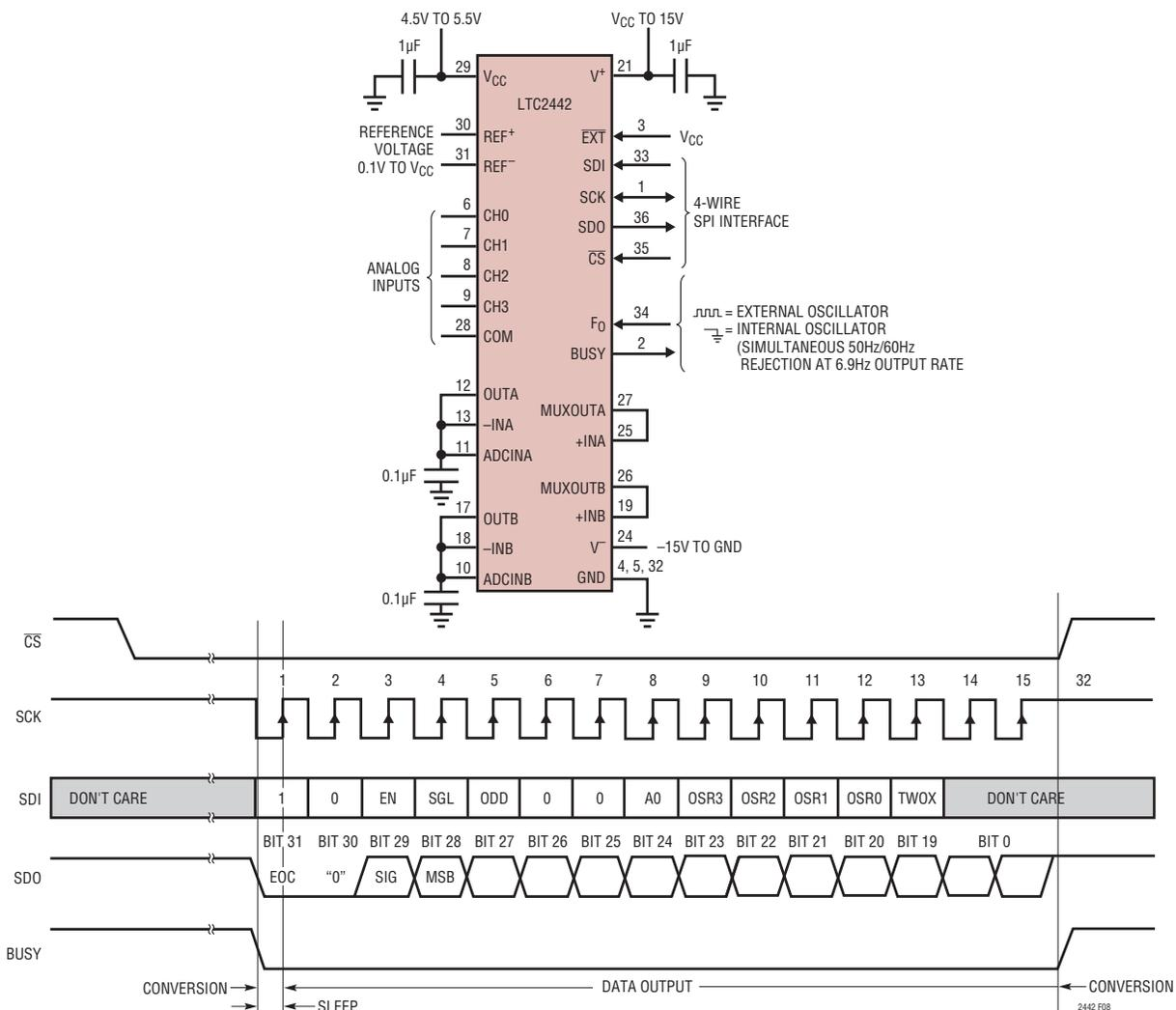
Figure 8. Internal Serial Clock, Reduced Data Output Length
