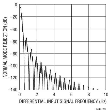
Figure 13. Normal Mode Rejection (Internal Oscillator at 90kHz)
