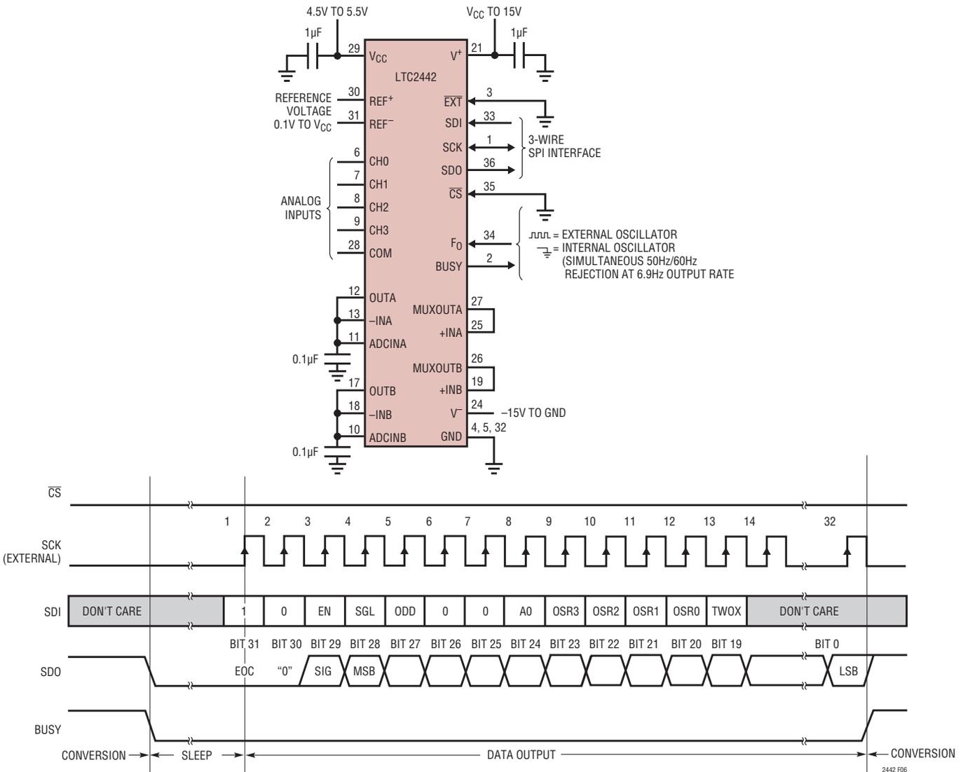
Figure 6. External Serial Clock,  $\overline{CS} = 0$  Operation (2-Wire)
