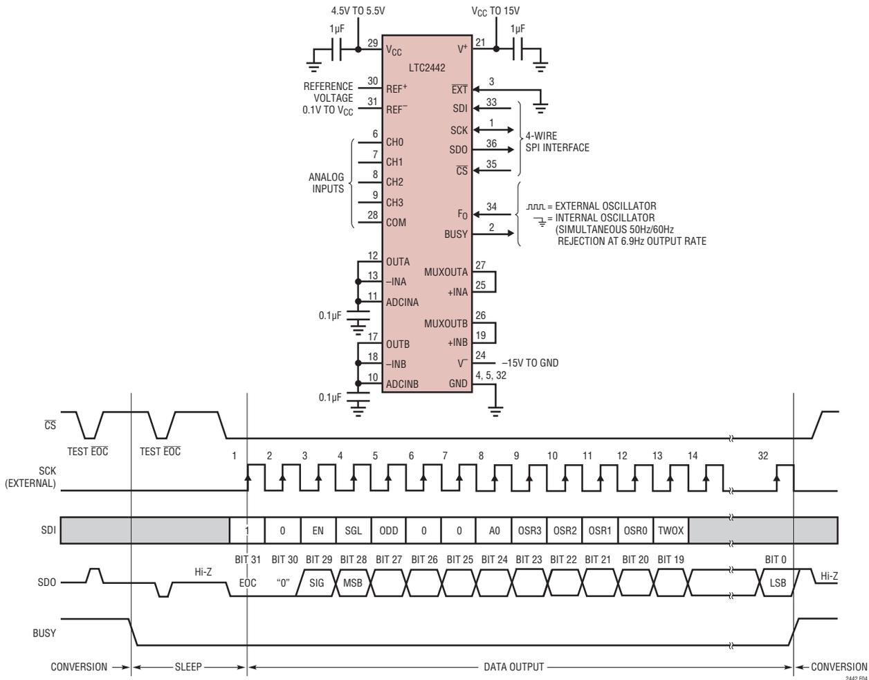
Figure 4. External Serial Clock, Single Cycle Operation
