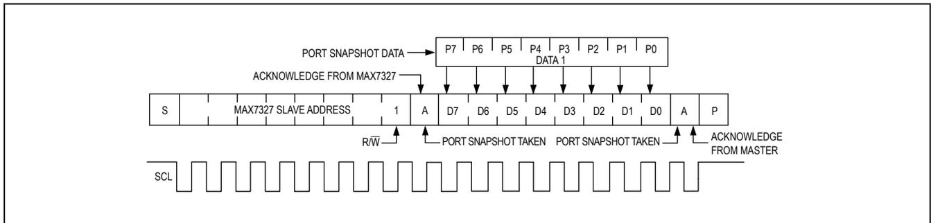
Figure 8. Reading Group B Ports of MAX7327
