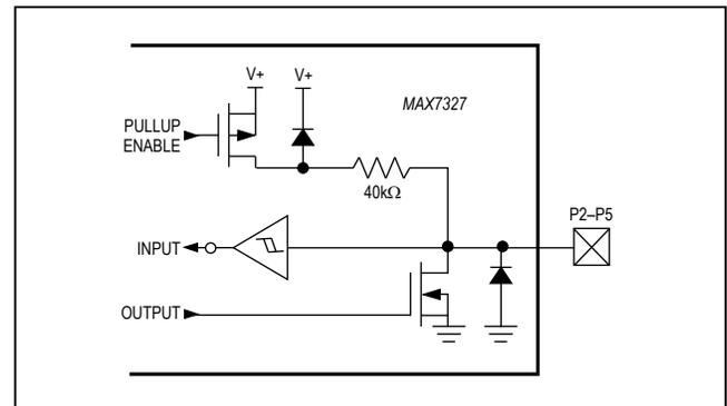
Figure 11. MAX7327 Open-Drain I/O Port Structure
