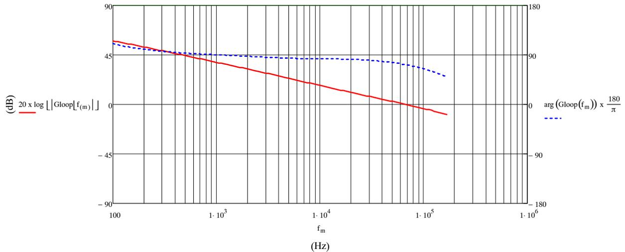
Figure 36. Bode Plot of the Total Loop
