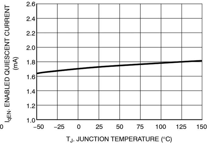
Figure 5. Enabled Quiescent Current vs. Junction Temperature
