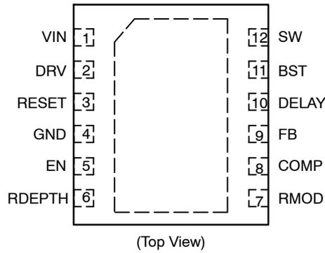
**Figure 3. Pin Connections**
