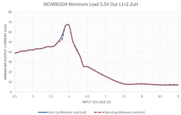
Typical Minimum Load 5.5 V Out,  $L_1 = 2.2 \mu\text{H}$
