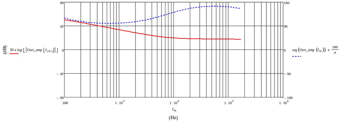
Figure 35. Bode Plot of the OTA Compensator
