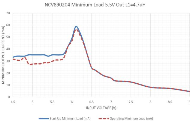
Typical Minimum Load 5.5 V Out,  $L_1 = 4.7 \mu\text{H}$
