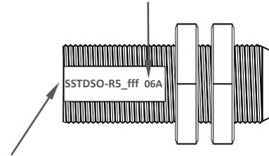
CHARACTERISTIC-OPTION\_TRIP SPEED MARKED ON THIS SURFACE
