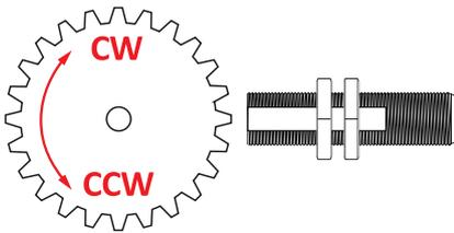
**THIS SENSOR WORKS WITH ANY ORIENTATION!**
