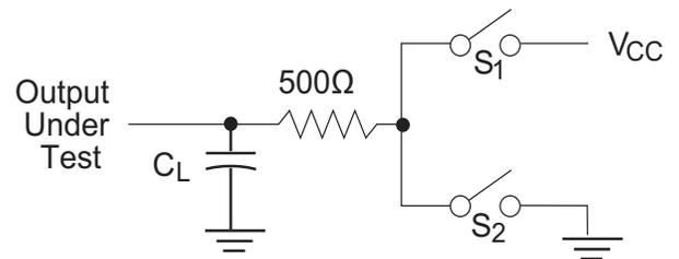
Figure 4: Driver Timing Test Load #2 Circuit
