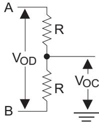
Figure 1: RS-485 Driver DC Test Load Circuit
