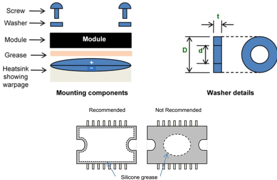
Figure 15. Module Mounting details : components ; washer drawing ; need for even spreading of thermal grease
