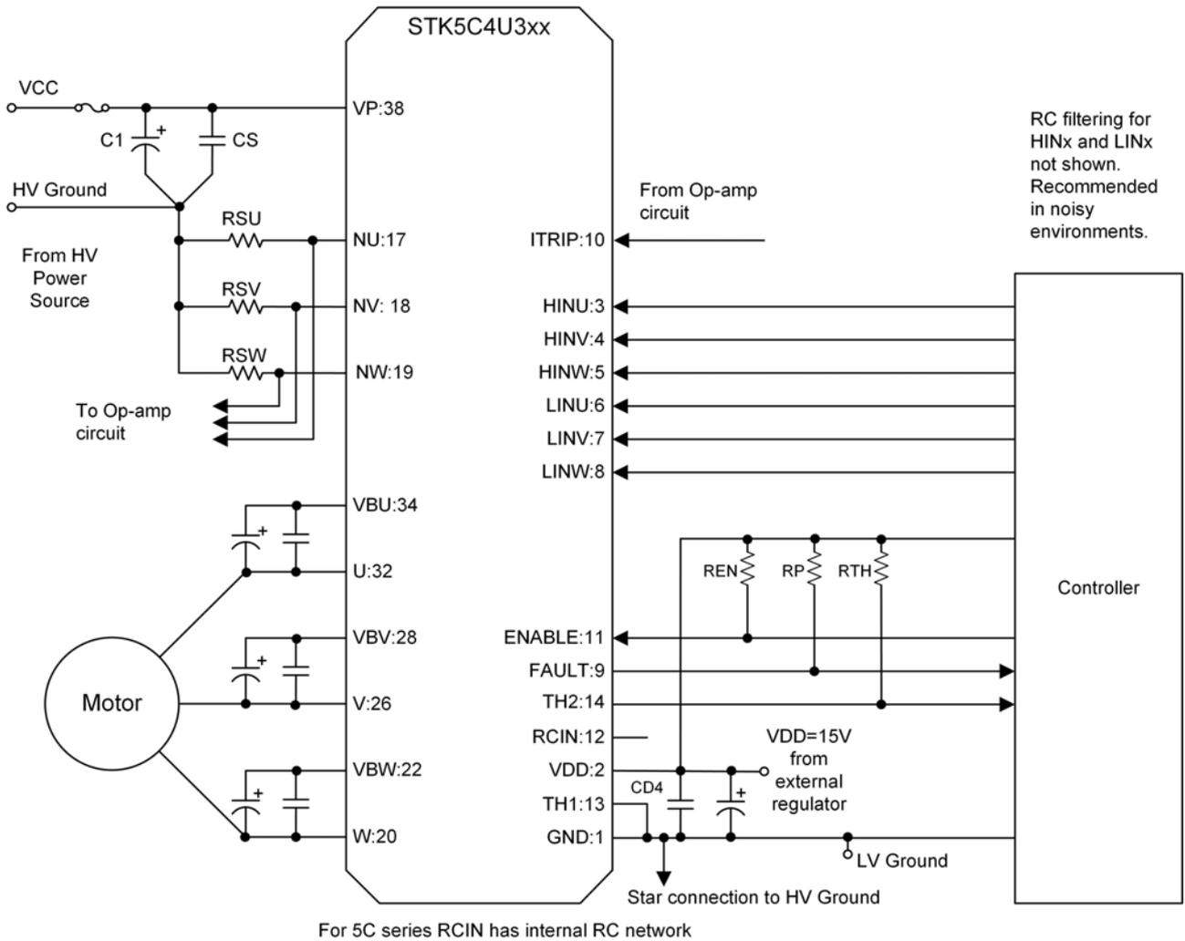
**Figure 2. Application Schematic**
