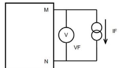
Figure 18. Test circuit for V<sub>F</sub>
