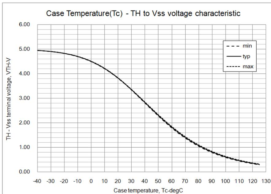
Figure 13. Thermistor Voltage versus Case Temperature
