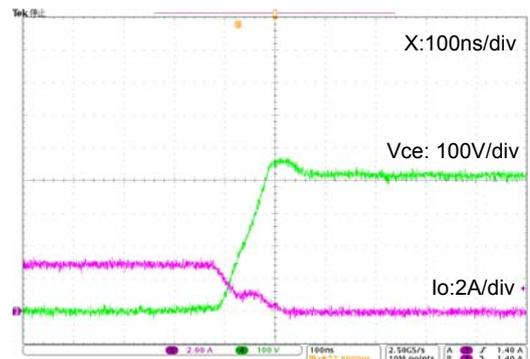
Figure 10. Turn-off waveform  $T_J = 100^\circ\text{C}$ ,  $V_{CC} = 400\text{ V}$
