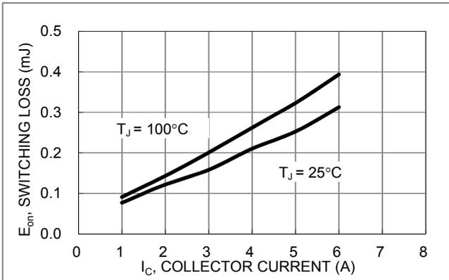
Figure 6.  $E_{ON}$  versus  $I_D$  for different temperatures
