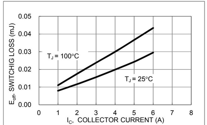
Figure 7.  $E_{OFF}$  versus  $I_D$  for different temperatures
