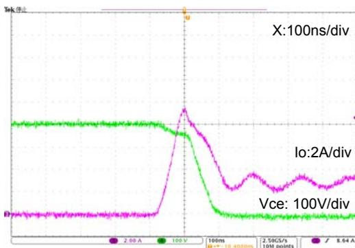
Figure 9. Turn-on waveform  $T_J = 100^\circ\text{C}$ ,  $V_{CC} = 400\text{ V}$
