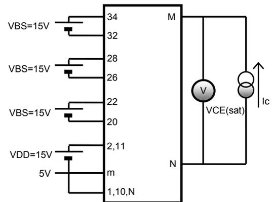
Figure 17. Test circuit for V<sub>CE(sat)</sub>
