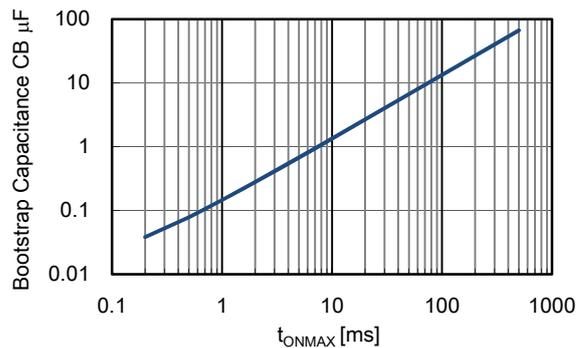
**Figure 14. Bootstrap capacitance versus t<sub>ONMAX</sub>**
