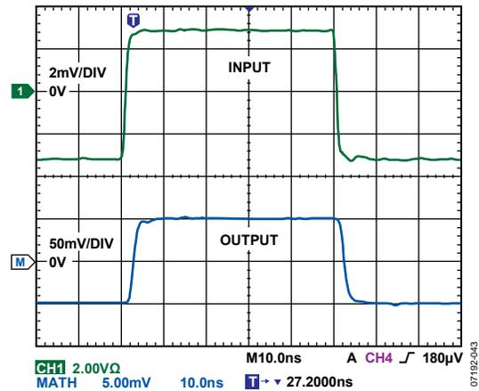
Figure 43. Small-Signal Pulse Response for the VGA/Preamplifier
