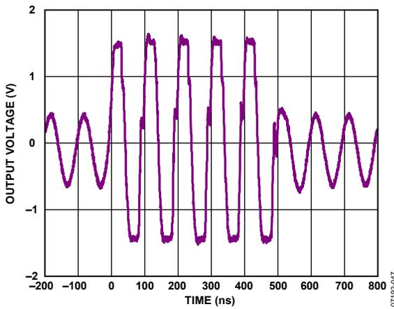
Figure 47. Overdrive Recovery of the VGA/Preamplifier—Gain Code = 1011
