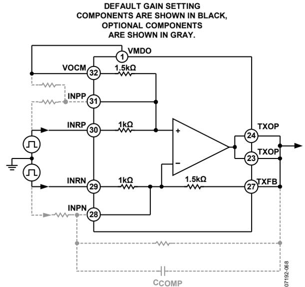
Figure 68. Gain-Setting Resistors of the High Current Driver
