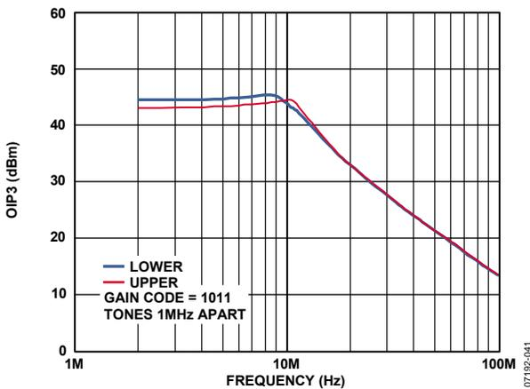
Figure 41. OIP3 vs. Frequency for the VGA/Preamplifier
