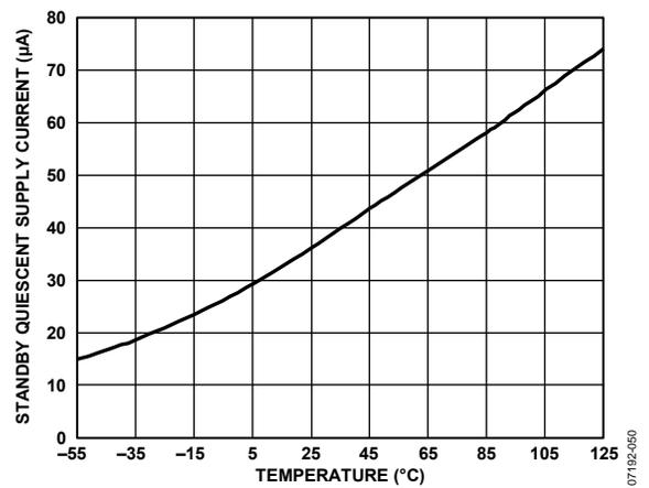
Figure 50. Standby Quiescent Supply Current vs. Temperature
