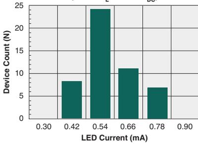
**Typical  $I_F$  for Switch Dropout**
