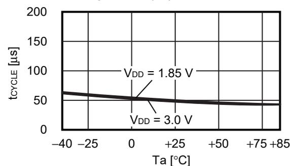
**2.6 Operating cycle ( $t_{CYCLE}$ ) vs. Power supply voltage ( $V_{DD}$ )**
