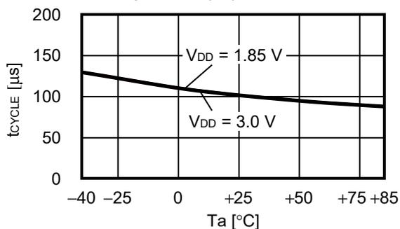
1.6 Operating cycle ( $t_{CYCLE}$ ) vs. Power supply voltage ( $V_{DD}$ )
