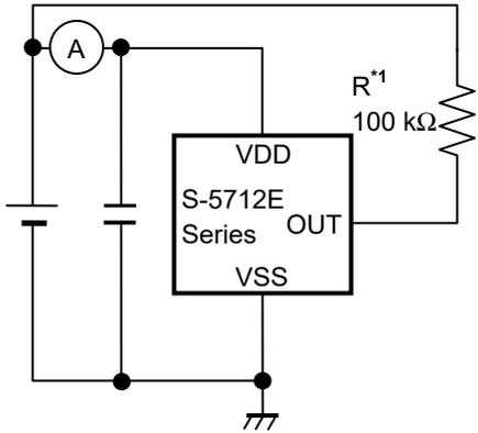
\*1. Resistor (R) is unnecessary for the CMOS output product.
