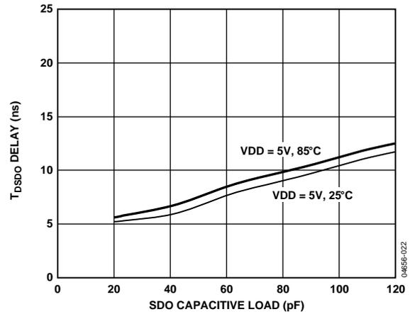
Figure 22.  $t_{SDO}$  Delay vs. Capacitance Load and Supply
