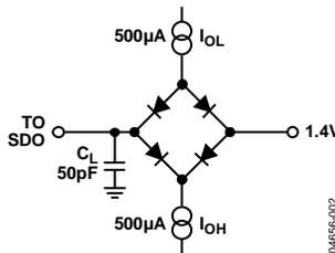
Figure 2. Load Circuit for Digital Interface Timing
