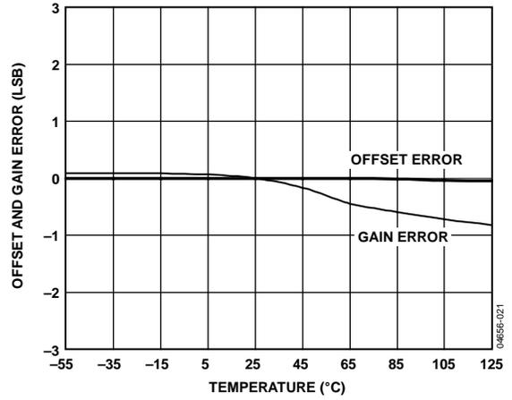
Figure 21. Offset and Gain Error vs. Temperature
