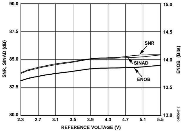
Figure 12. SNR, SINAD, and ENOB vs. Reference Voltage
