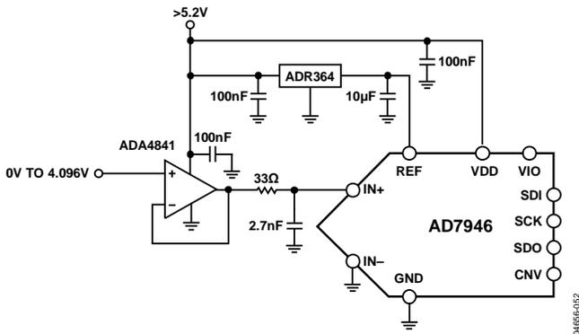
Figure 32. Example of a Single-Supply Application Circuit
