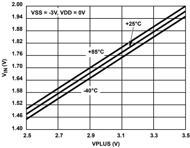
FIGURE 29. DIGITAL SWITCHING POINT vs SUPPLY VOLTAGE
