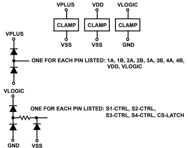
FIGURE 7. ESD/OVERVOLTAGE PROTECTION
