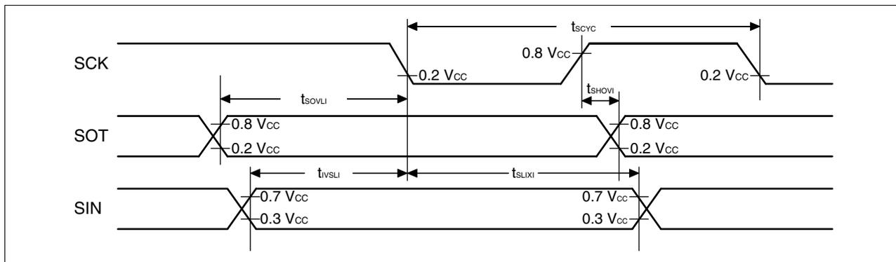
Sampling is executed at the falling edge of the sampling clock\*<sup>1</sup>, and serial clock delay is enabled\*<sup>2</sup>.
