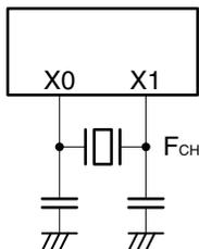
When an external clock is used (X1 is open)
