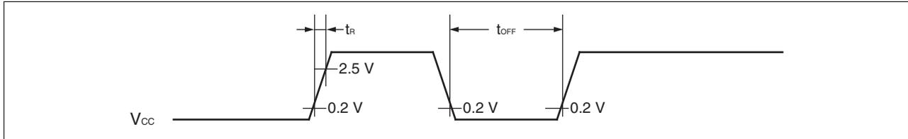
Note: A sudden change of power supply voltage may activate the power-on reset function. When changing the power supply voltage during the operation, set the slope of rising to a value below within 30 mV/ms as shown below.
