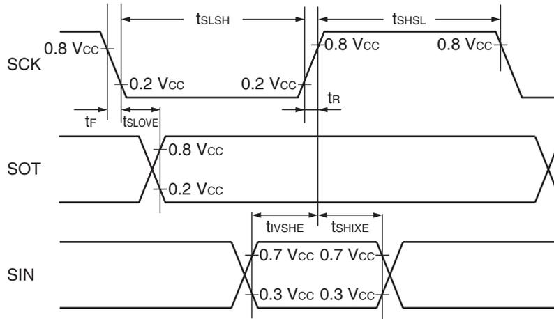
Sampling is executed at the falling edge of the sampling clock\*<sup>1</sup>, and serial clock delay is disabled\*<sup>2</sup>.
