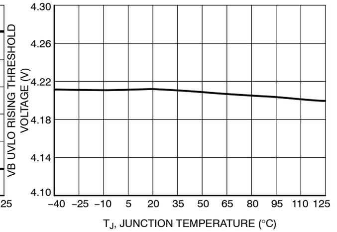
Figure 16. VB UVLO Rising Threshold vs. Junction Temperature
