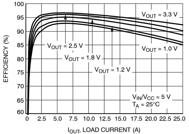
Figure 14. Efficiency vs.  $I_{out}$
