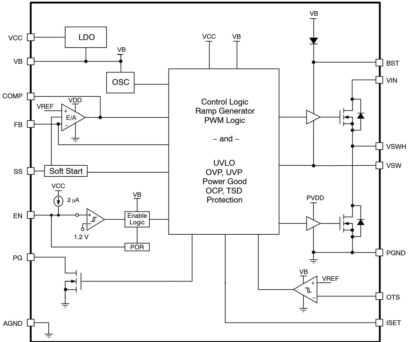
Figure 1. NCP3231A Block Diagram
