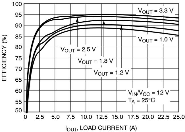
Figure 13. Efficiency vs.  $I_{out}$
