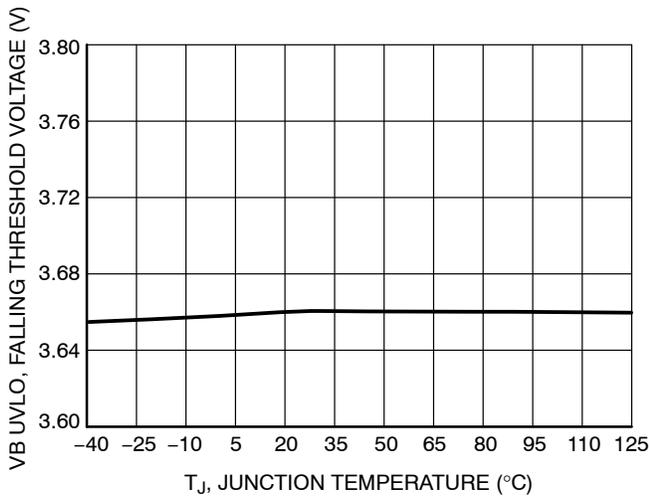
Figure 17. VB UVLO Falling Threshold vs. Junction Temperature
