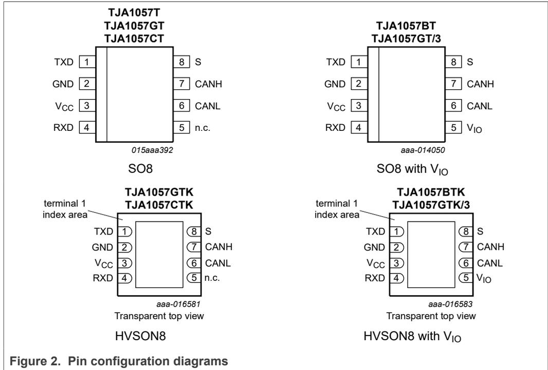
Figure 2. Pin configuration diagrams
