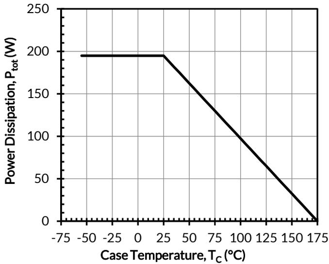
Figure 15. Total power dissipation
