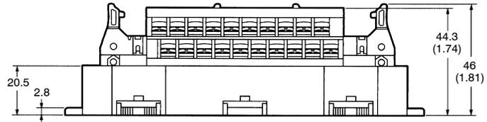
Note: The terminal block has a terminal pitch of 7.62 mm.
