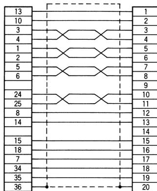
For W-Series Servo Driver and Servo Terminal Block
