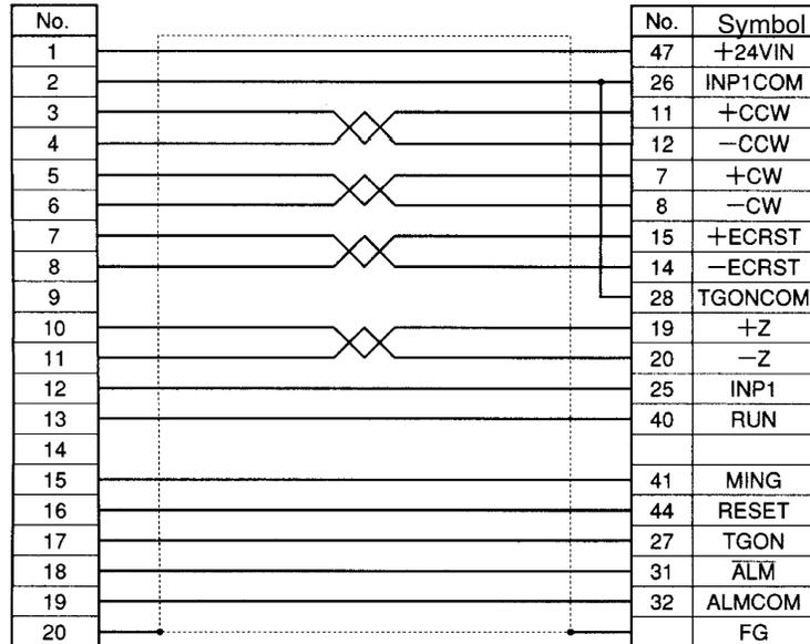
Cable: AWG28 × 4P + AWG28 × 9C
