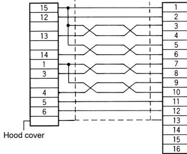
**For U-Series Servo Driver and Servo Terminal Block**
