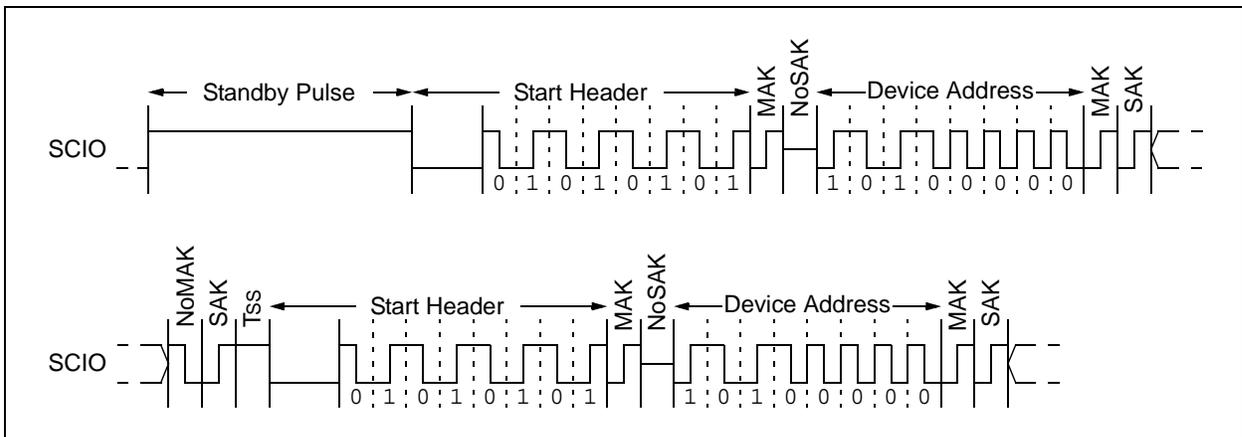
Upon detection of the standby pulse, a slave device will typically enter its lowest power state. The exception to this is when the slave device is executing an internal process in the background. Examples include an EEPROM performing a write cycle, or a temperature sensor carrying out a conversion.
