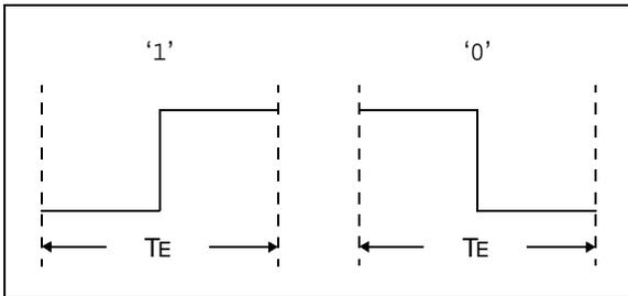
Because every bit period must have a middle edge transition, there may or may not exist another edge transition at the beginning of a bit period. This is entirely dependent upon the values of both the previous and current bits. If two bits of equal value are being successively transmitted, then a transition at the beginning of the second bit is required. If the two bits are of opposing values, then no edge will occur. Refer to Figure 4-2 for details.
