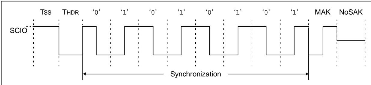
During the Acknowledge sequence following the start header, no slave device will respond with a SAK. Within this time, the bus will not be driven by any device and no edge transition will occur. Refer to **Section 5.1 "Acknowledge Sequence"** for details.
