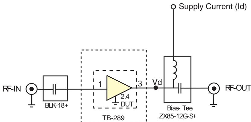
**Fig 1.** Block Diagram of Test Circuit used for characterization. (DUT soldered on Mini-Circuits Characterization test board TB-289) Gain, Return loss, Output power at 1dB compression (P1 dB) , output IP3 (OIP3) and noise figure measured using Agilent’s N5242A PNA-X microwave network analyzer.
