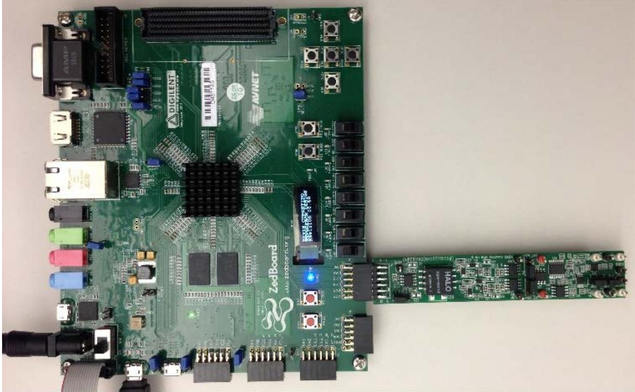
Figure 1. Santa Fe Board Connected to ZedBoard Development Kit
