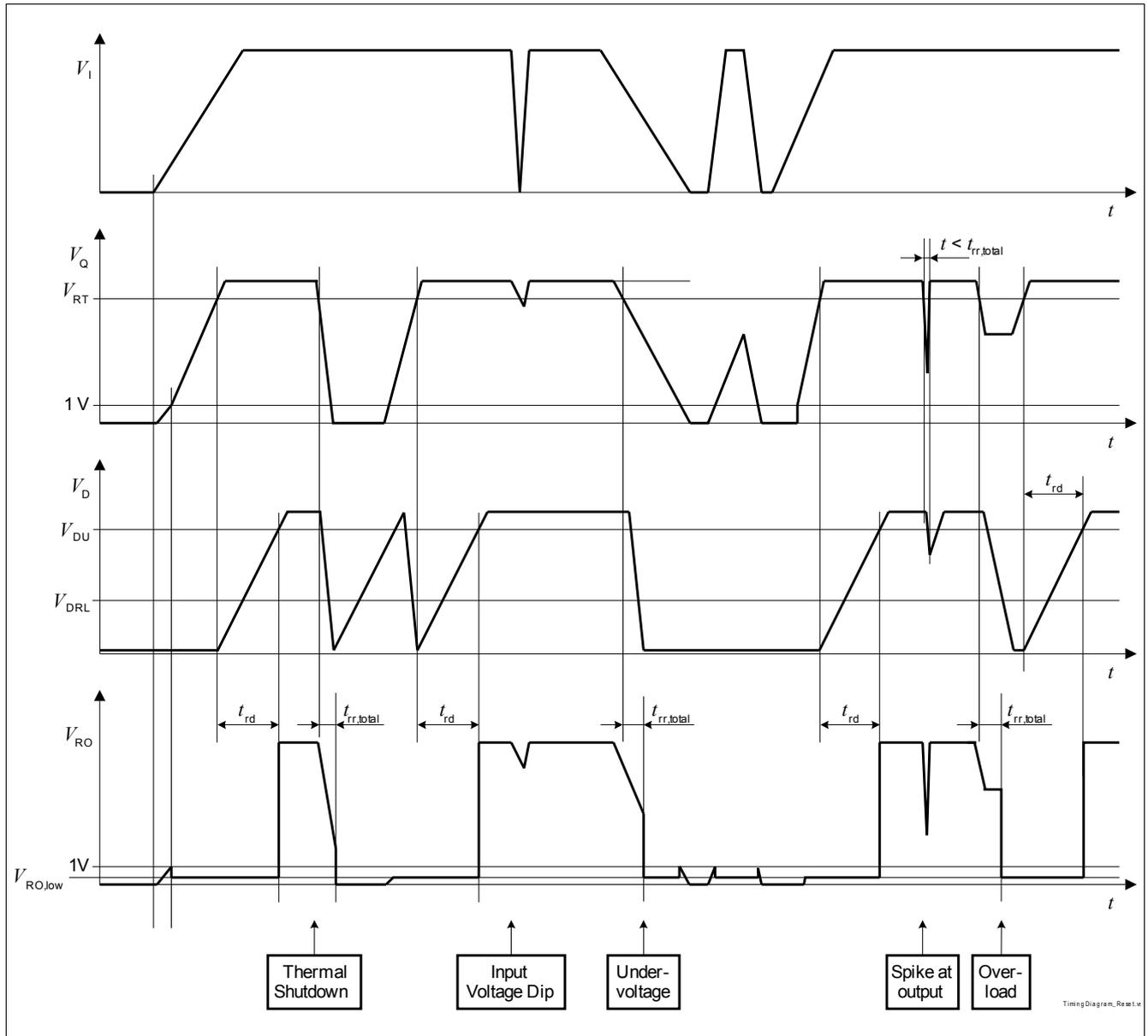
**Figure 6 Timing diagram reset**
