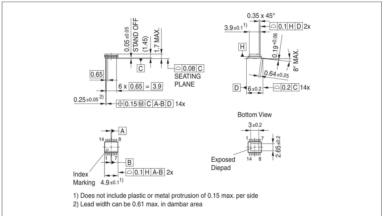
**Figure 11 PG-SSOP-14 Exposed Pad<sup>1)</sup>**
