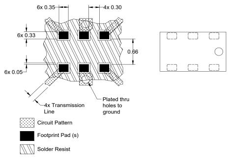
Dimensions are in Millimeters Mounting Footprint
