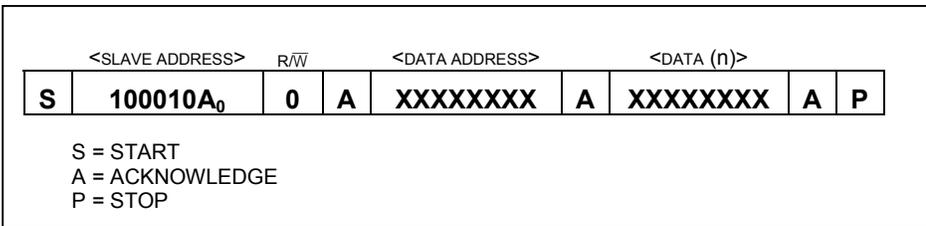
**Figure 5. Data Read—Slave Transmitter Mode**
