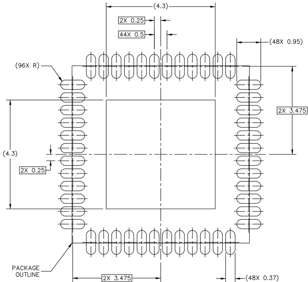
PCB DESIGN GUIDELINES – SOLDER MASK OPENING PATTERN
