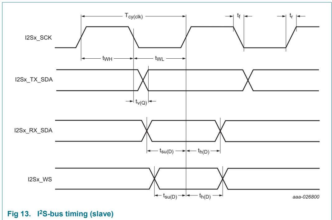
Fig 13. I<sup>2</sup>S-bus timing (slave)
