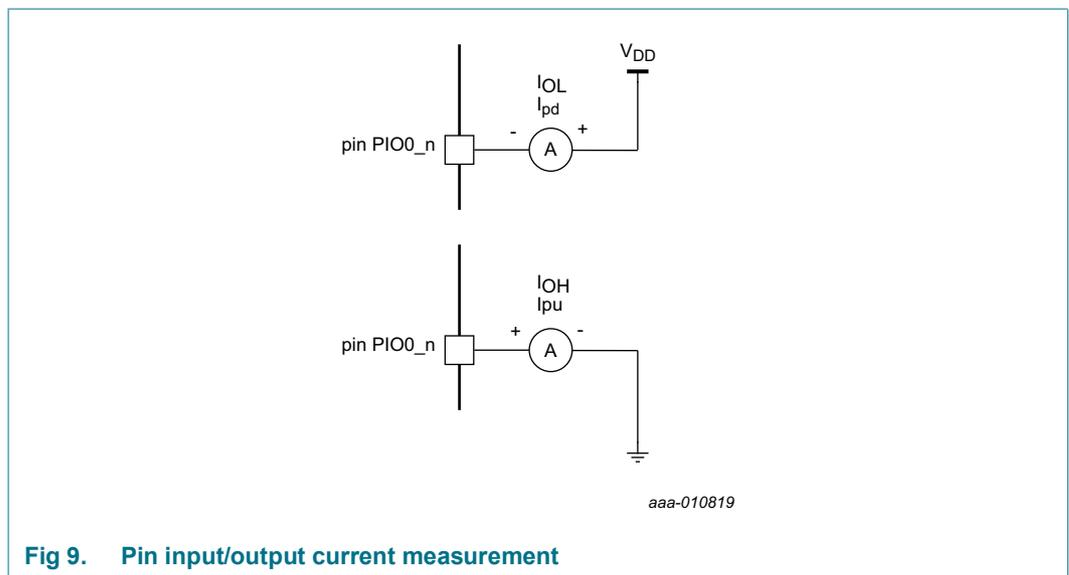
**Fig 9. Pin input/output current measurement**
