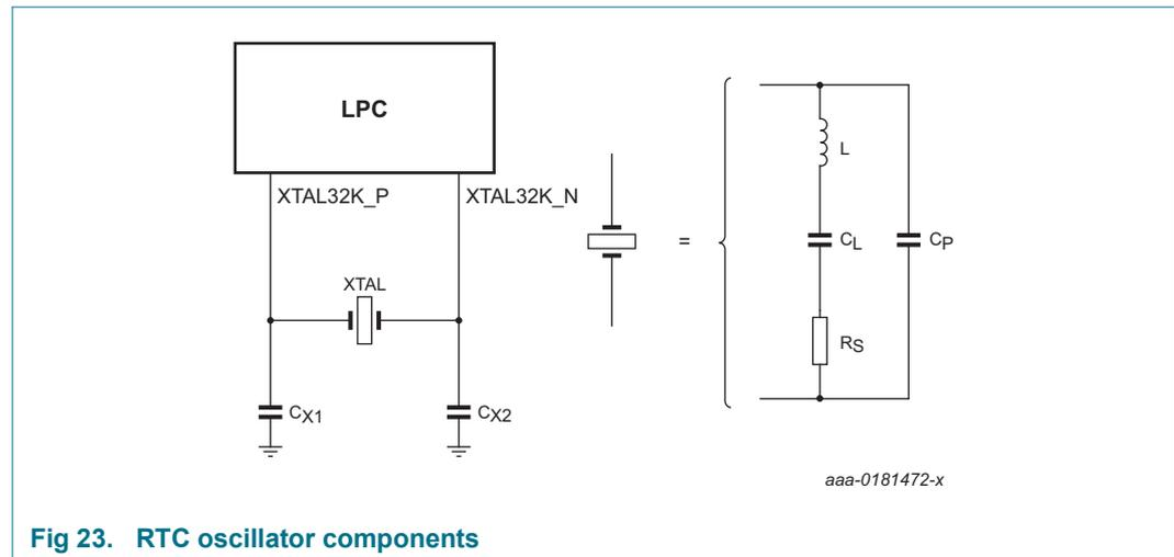
**Fig 23. RTC oscillator components**
