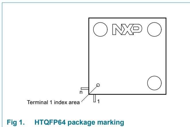
The LPC55S0x/LPC550x HTQFP64 package has the following top-side marking:
