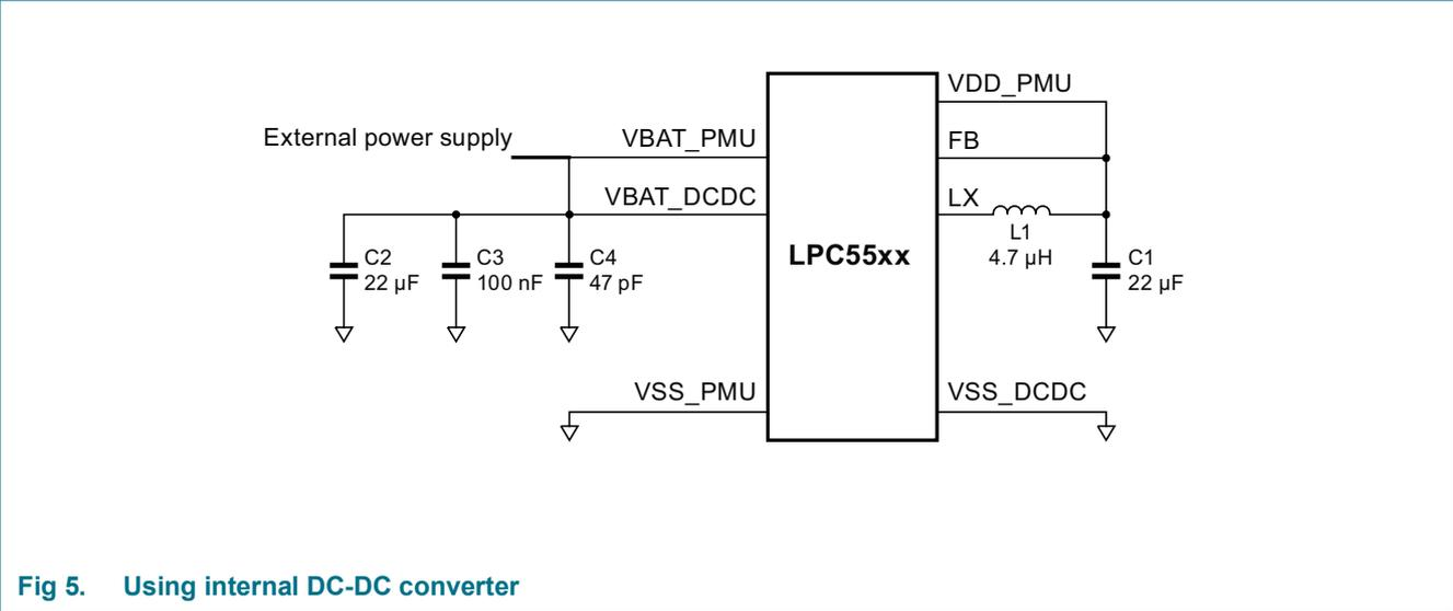
Fig 5. Using internal DC-DC converter
