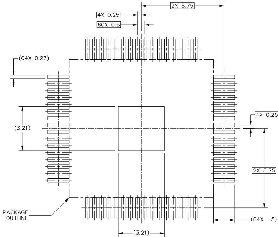
PCB DESIGN GUIDELINES – I/O PADS AND SOLDERABLE AREA
