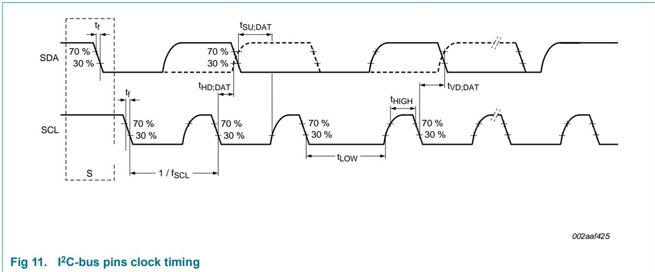
Fig 11. I<sup>2</sup>C-bus pins clock timing
