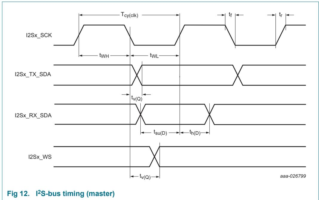
Fig 12. I<sup>2</sup>S-bus timing (master)
