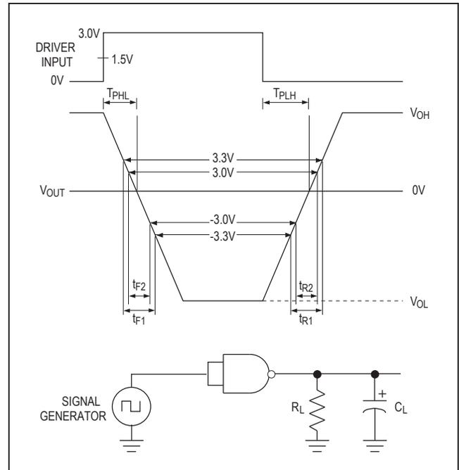
Figure 1. Slew-Rate Test Circuit and Timing Diagram
