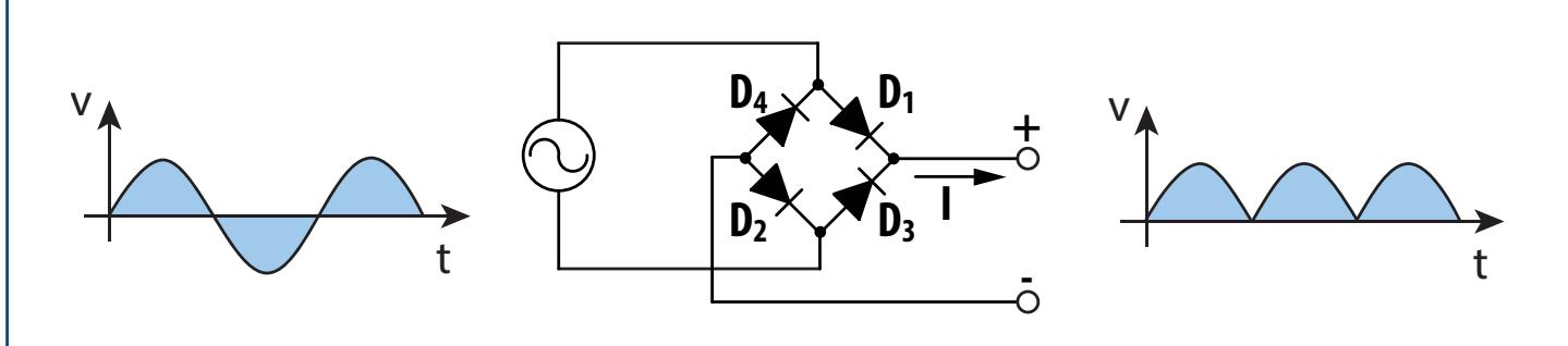
A bridge rectifier diode or four discrete rectifier diodes connected in a closed loop "bridge" configuration provide full-wave rectification from AC input into a DC output. The bridge rectifier diode blocks the current in the reverse direction and allows the current in the forward direction to keep the output current in one direction. During the
