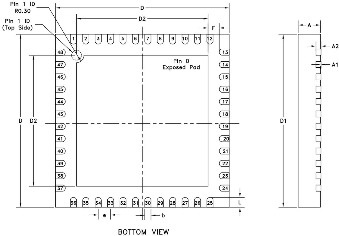
**Table 26: 7x7 mm QFN 48 Pin (LP7) Dimensions**
