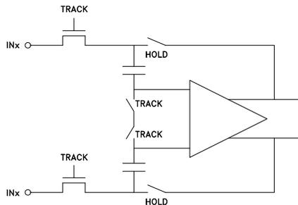
Figure 11: Input configuration
