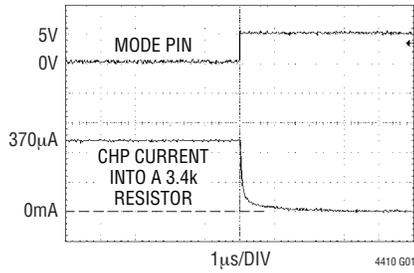
**CHP Current with I<sub>LOAD</sub> Step**
