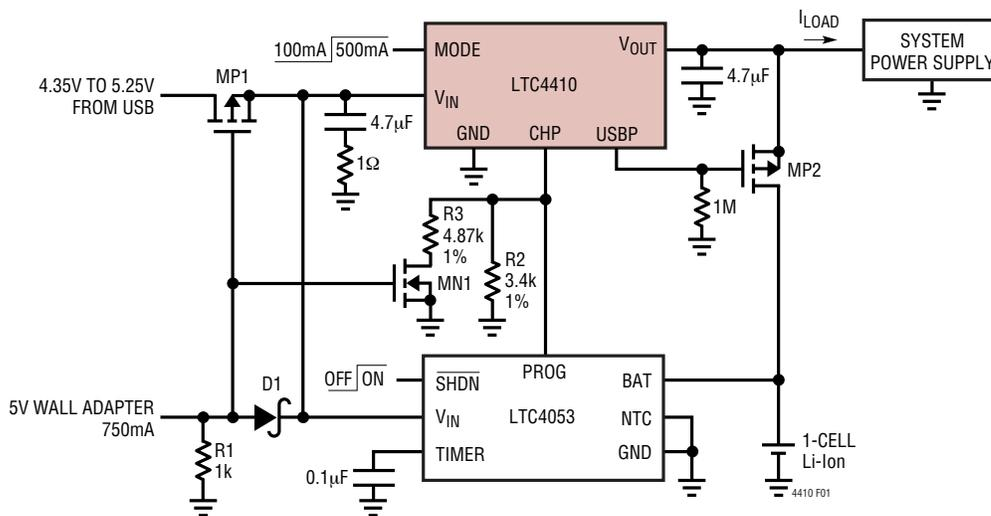
Figure 1. USB Power Management and Wall Adapter Power
