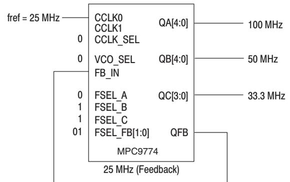
MPC9774 example configuration (feedback of QFB = 25 MHz, VCO\_SEL = +2, M = 8, N<sub>A</sub> = 2, N<sub>B</sub> = 4, N<sub>C</sub> = 6, f<sub>VCO</sub> = 400 MHz).
