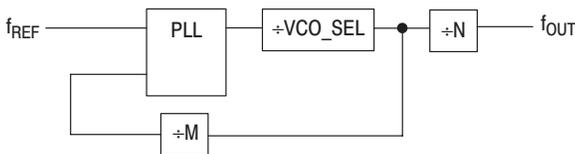
where  $f_{REF}$  is the reference frequency of the selected input clock source (CCLK0 or CCLK1), M is the PLL feedback divider and N is a output divider. M is configured by the FSEL\_FB[0:1] and N is individually configured for each output bank by the FSEL\_A, FSEL\_B and FSEL\_C inputs.
