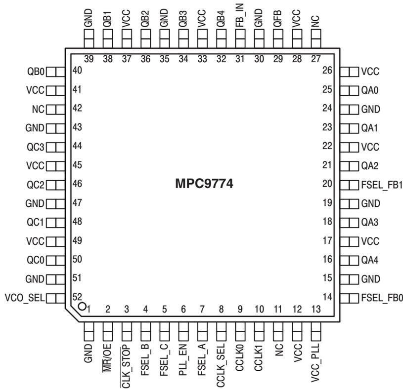
Figure 2. MPC9774 52-Lead Package Pinout (Top View)
