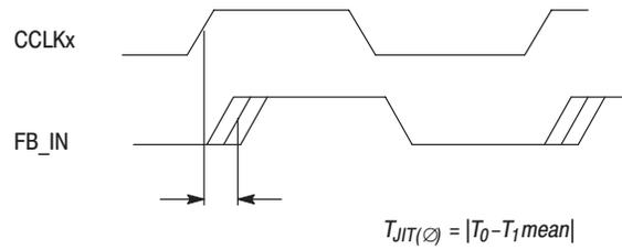
The deviation in  $t_0$  for a controlled edge with respect to a  $t_0$  mean in a random sample of cycles
