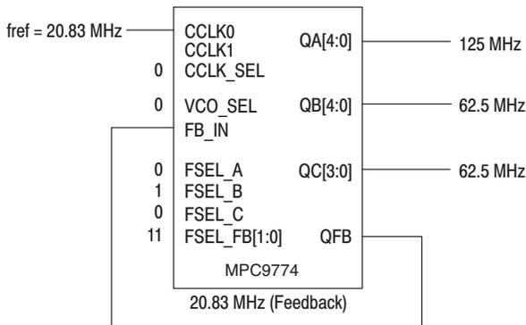
MPC9774 example configuration (feedback of QFB = 20.83 MHz, VCO\_SEL = +2, M = 12, N<sub>A</sub> = 2, N<sub>B</sub> = 4, N<sub>C</sub> = 4, f<sub>VCO</sub> = 500 MHz).
