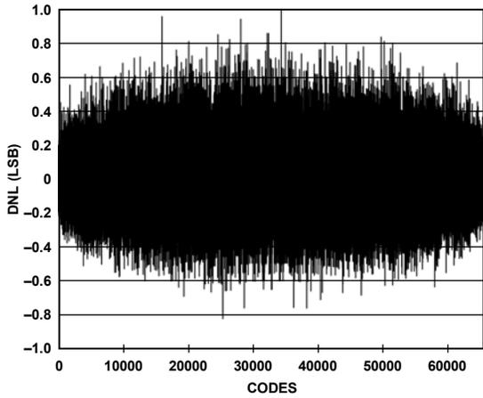
Figure 37. DNL with Dither Off,  $f_{IN} = 30$  MHz
