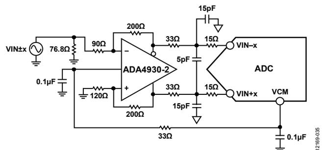
Figure 53. Differential Input Configuration Using the ADA4930-2
