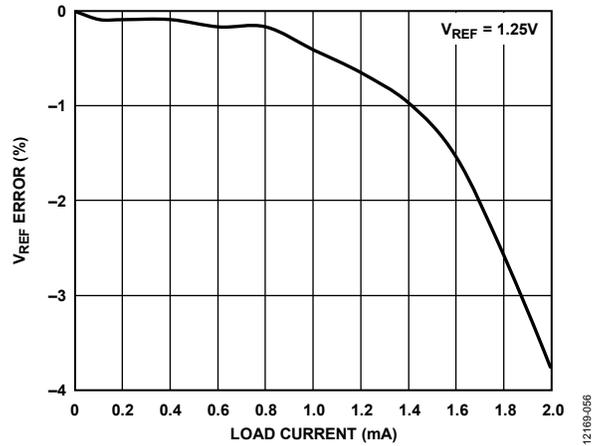
Figure 58. Reference Voltage Error vs. Load Current
