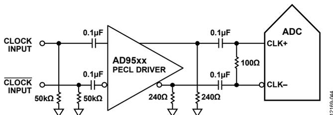
Figure 62. Differential PECL Sample Clock (Up to 1240 MHz)
