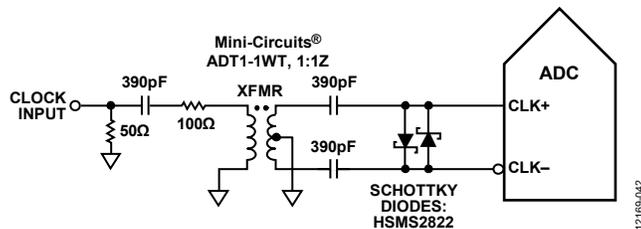
Figure 60. Transformer-Coupled Differential Clock (Up to 200 MHz)
