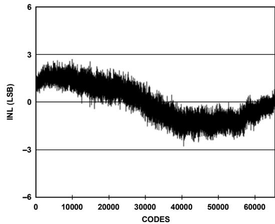
Figure 41. INL with Dither On,  $f_{IN} = 30$  MHz
