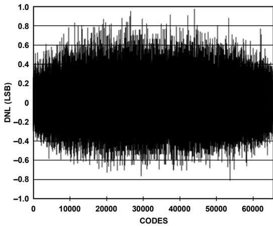
Figure 38. DNL with Dither On,  $f_{IN} = 30$  MHz
