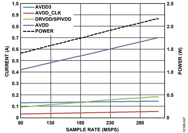
Figure 65. Power and Current vs. Sample Rate
