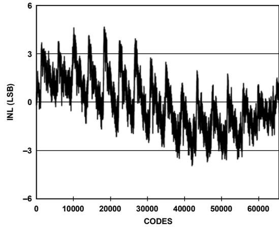
Figure 40. INL with Dither Off,  $f_{IN} = 30$  MHz
