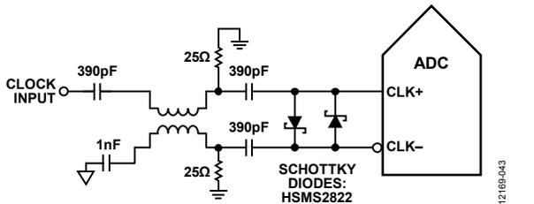
Figure 61. Balun-Coupled Differential Clock (Up to 1240 MHz)
