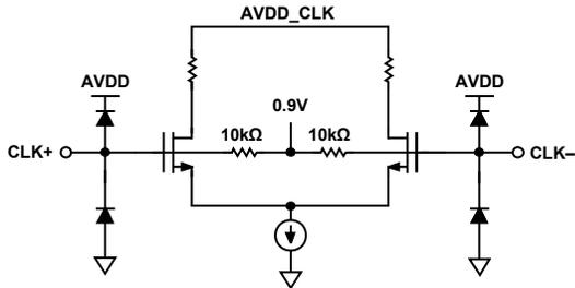
Figure 43. Equivalent Clock Circuit
